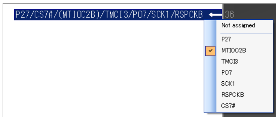
Figure 3.20 Pin function selection
