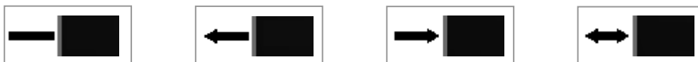
a. Pin function is not assigned b. Output c. Input d. Input/Output
