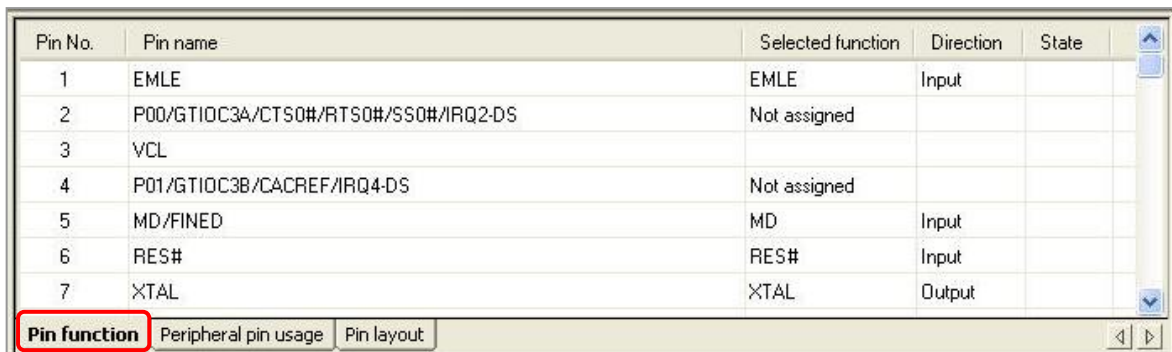
Figure 3.3 Pin-Function Pane ([Pin function] Sheet)
