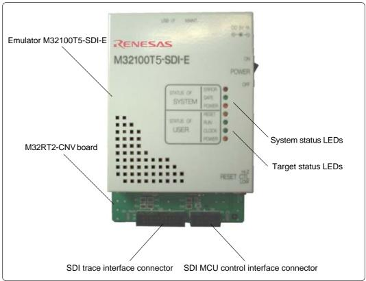
Figure 2.3 Name of each part on the upper panel
