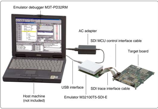
Figure 2.1 System configuration (JTAG connection)
