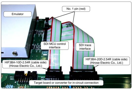
Figure 3.4 Connecting the SDI interface cables
