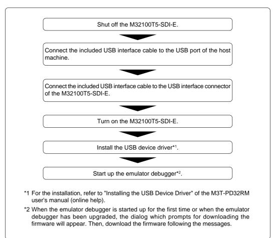
Figure 3.3 USB interface connection procedure
