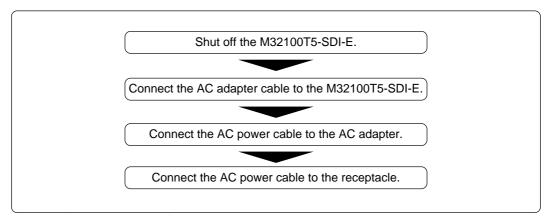
Figure 3.2 Connecting AC adapter
