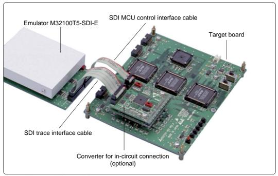
Figure 2.2 Magnified view of the in-circuit connection
