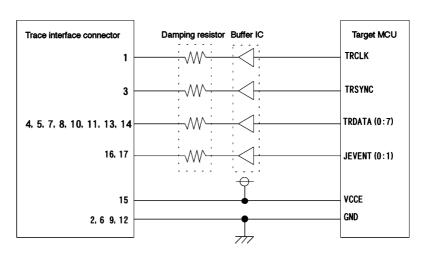
You can connect the signal lines of the SDI trace interface from the target MCU to the connector directly. However, to ensure safe operation of the emulator, insertion of a buffer IC and damping resistor to each signal line is recommended.
