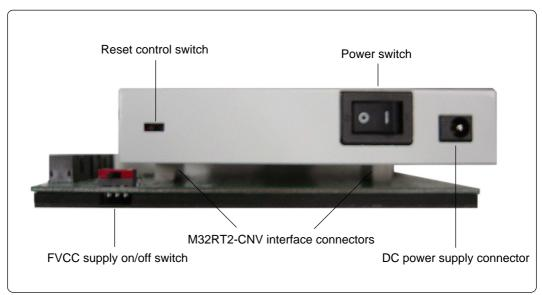
Figure 2.4 Name of each part on the side panel
