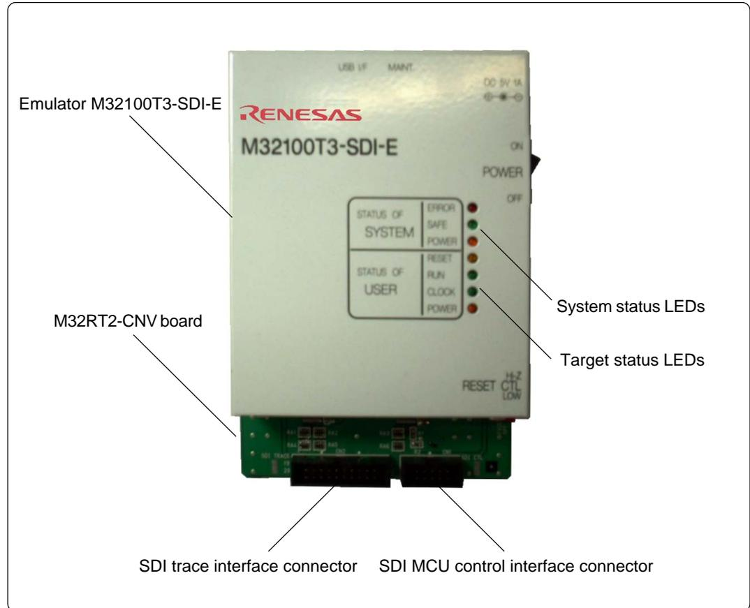
Figure 2.3 Name of each part on the upper panel
