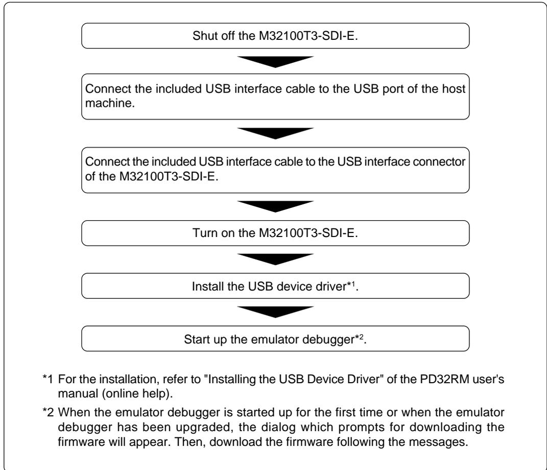
Figure 3.3 USB interface connection procedure
