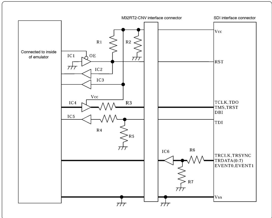
Figure 3.7 Circuit diagram of the emulator side of the SDI interface
