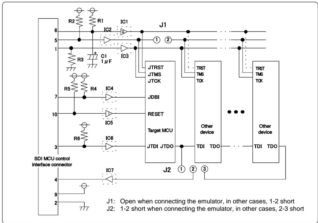
Figure 3.5 Sample circuit of the SDI MCU control interface
