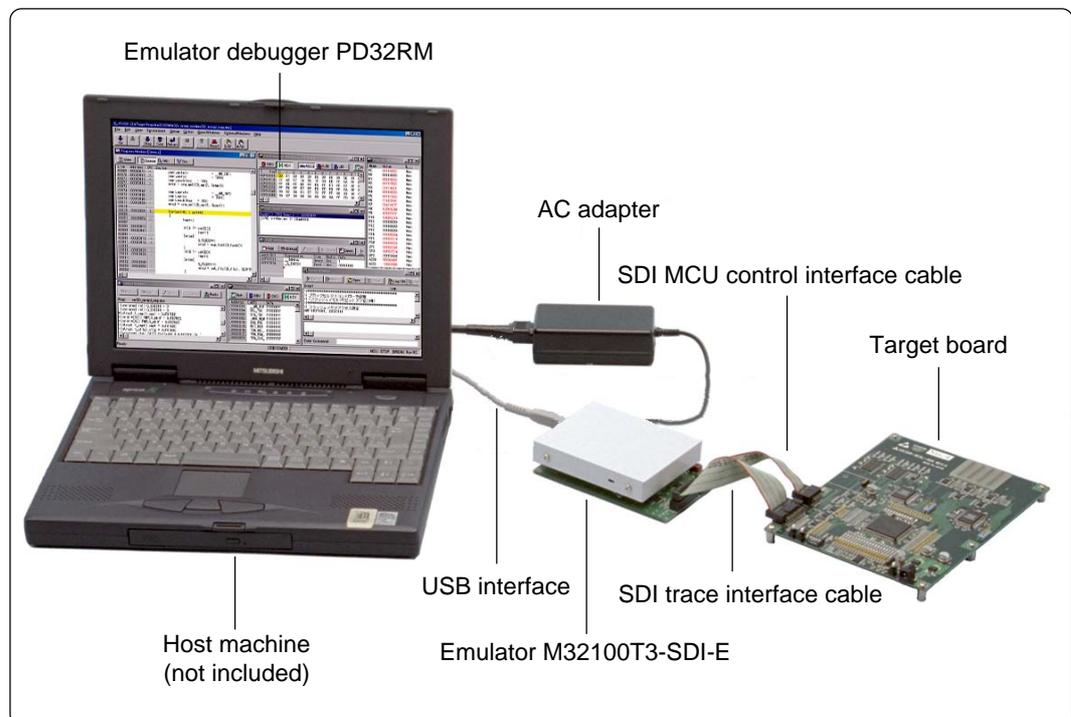
Figure 2.1 System configuration (JTAG connection)
