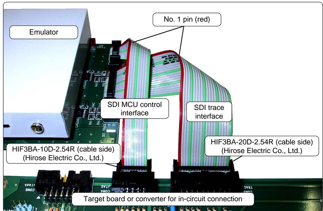
Figure 3.4 Connecting the SDI interface cables
