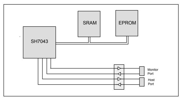
Figure 1.2 LCEVB-SH2 Functional Block Diagram
