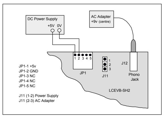
Figure 2.1 Power Supply Connection to LCEVB-SH2
