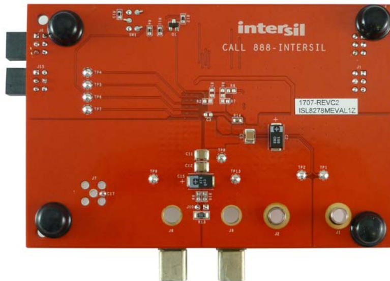
Figure 3. ISL8278MEVAL1Z Evaluation Board (Bottom Side)
