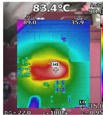
Figure 15. Thermal Image, 12V_{IN} to 1V_{OUT} , I_{OUT} = 33A , T_A = +25^\circ C , f_{SW} = 550kHz , No Air Flow
