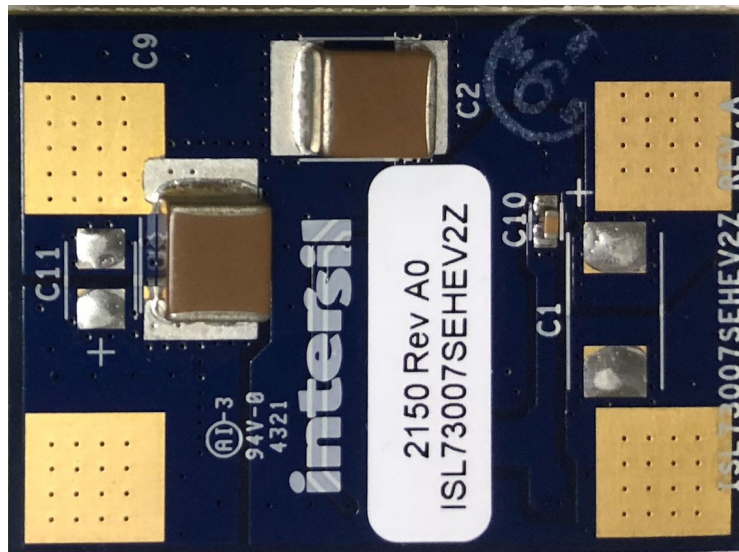
Figure 4. ISL73007SEHEV2Z Evaluation Board (Bottom)
