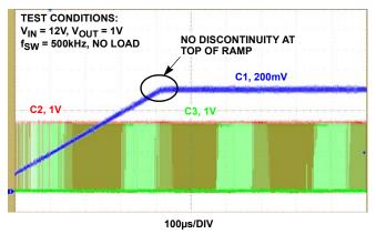
FIGURE 15. SOFT-START RAMP COMPLETION
