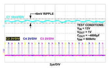
FIGURE 12.  $V_{OUT}$  RIPPLE, 3-PHASE INTERLEAVE
