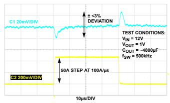
FIGURE 11. DYNAMIC LOAD STEP, 0A TO 50A, di/dt = 100A/µs
