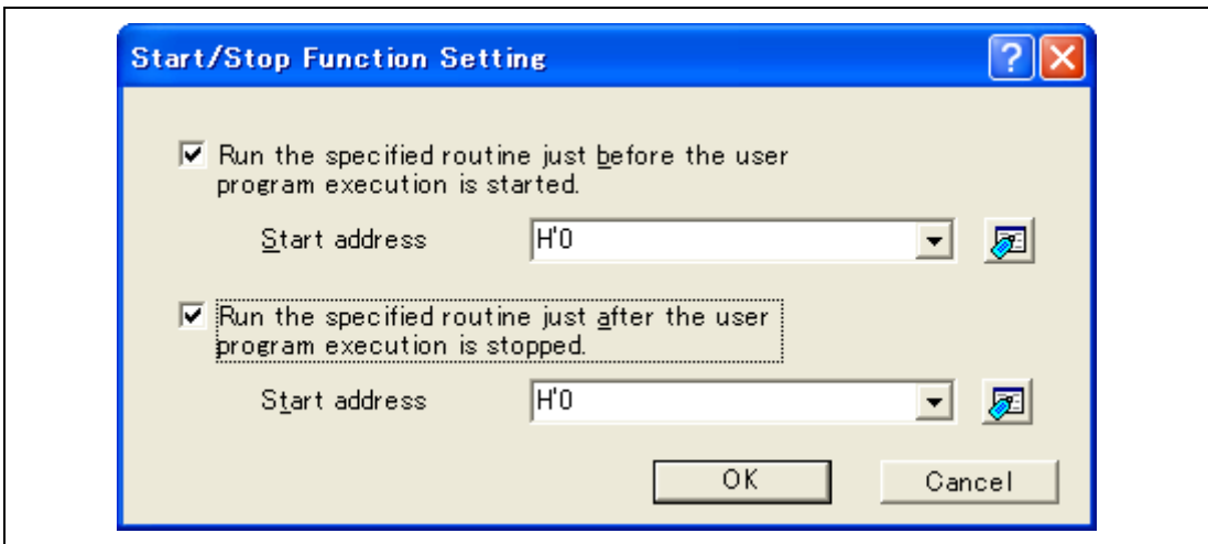
Figure 5.15 [Start/Stop Function Setting] Dialog Box
