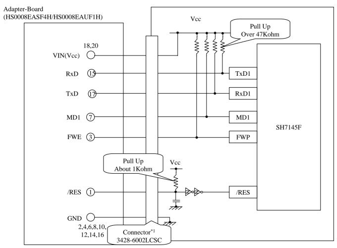
Setting the switches on the HS0008EASF4H on using SH7145F
