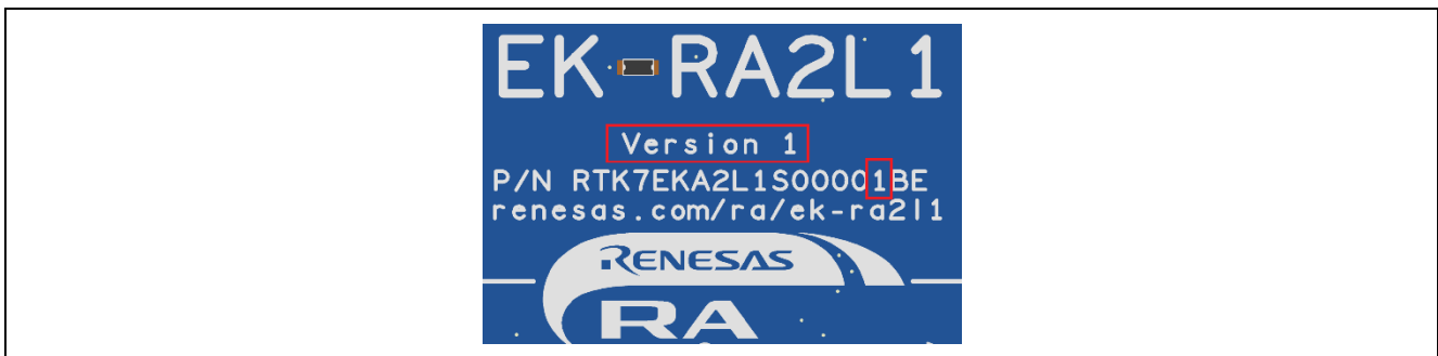
Figure 5. Identification of the Kit Version Number on the EK-RA2L1 Board
