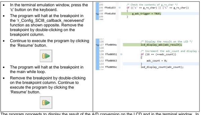
The program proceeds to display the result of the A/D conversion on the LCD and in the terminal window. In addition, the running count of A/D conversions performed is displayed in binary form using LEDs 0-3 on the RSK+. Adjust the potentiometer and press SW1, SW2 or SW3 on the RSK+ and an additional A/D conversion will be performed.
