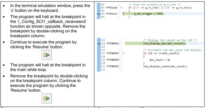
The program proceeds to display the result of the A/D conversion on the LCD and in the terminal window. In addition, the running count of A/D conversions performed is displayed in binary form using LEDs 0-3 on the RSK. Adjust the potentiometer and press SW1, SW2 or SW3 on the RSK and an additional A/D conversion will be performed.
