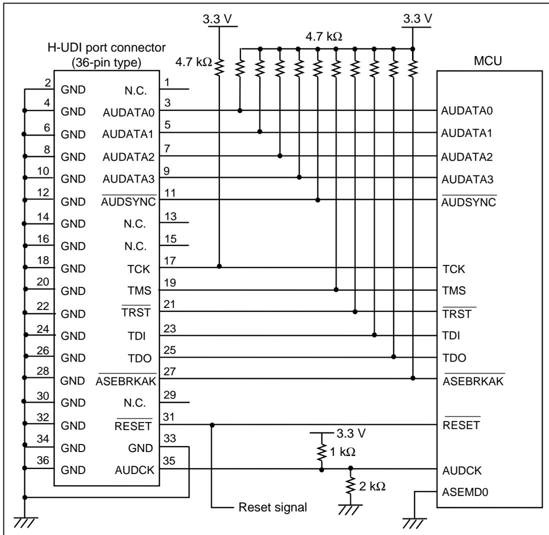
**Figure 4.1 Recommended Circuit for Connection between the H-UDI Port Connector and the MCU when Using the Emulator (36-Pin Type)**
