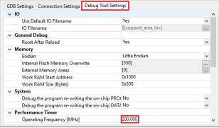
Figure 6-3 Debug Tool Settings
