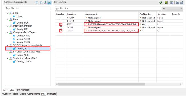
Figure 4-44 Configure pin assignment - Config\_SCI11
