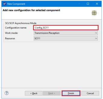
Figure 4-30 Ensure Configuration name - Config\_SCI11
