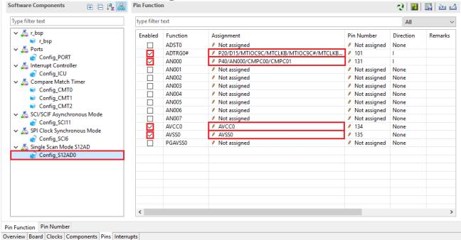
Figure 4-46 Configure pin assignment - Config\_S12AD0
