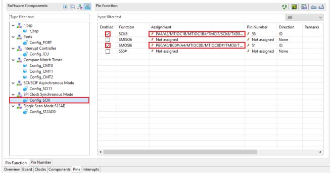
Figure 4-45 Configure pin assignment - Config\_SCI6
