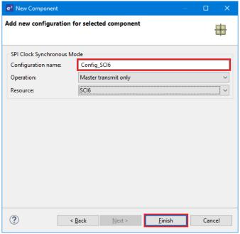
Figure 4-35 Ensure Configuration name - Config\_SCI6
