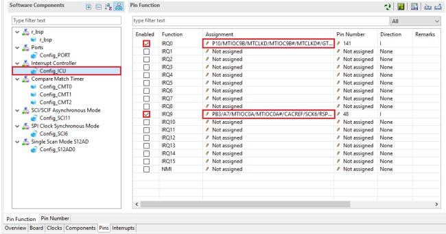
Figure 4-43 Configure pin assignment - Config ICU
