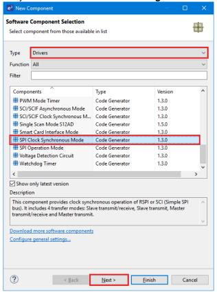
Figure 4-32 Select SPI Clock Synchronous Mode
