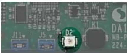
Figure 33: LED D2 on ProDK
