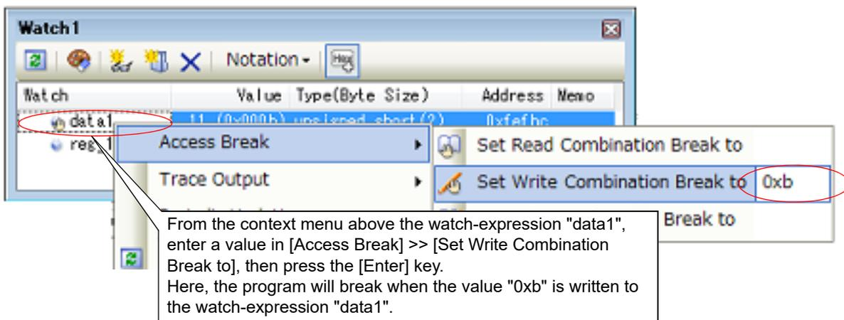
When you have performed the above operation, the set break event (access type) is managed in the [Events panel](#) as a Hardware Break event (access type) or a execution-related event in the detailed information on a Combination Break event (see "2.16 Manage Events" for details).
