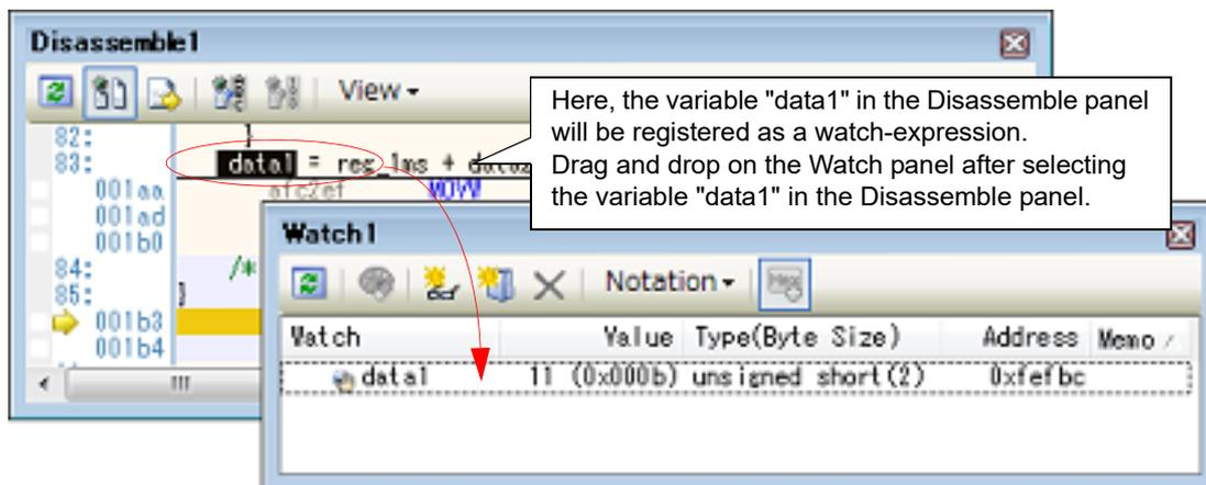
Remark You can also add a watch-expression by doing the following. First, select the target for which you wish to register a watch-expression, or move the caret to one of the target strings (the target is determined automatically). Next, from the context menu, select [Register Watch1] (but this is limited to the Watch panel (Watch 1)).
