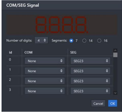
Enter the desired number of digits, number of segment and select the control signals for the individual segments. Click on the [OK] button to complete the settings.
