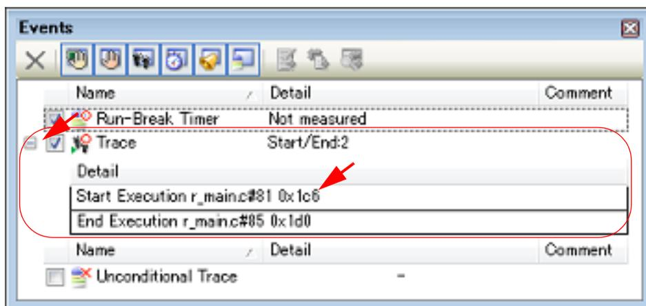
Remark 1. If either one of a trace start event and a trace end event is set as [Valid state](#), the check box of Unconditional Trace event in the [Events panel](#) is automatically cleared, therefore, trace data collection does not automatically start with the start of the program execution (the tracer will not run until the condition of the trace start event that has been set is met).
