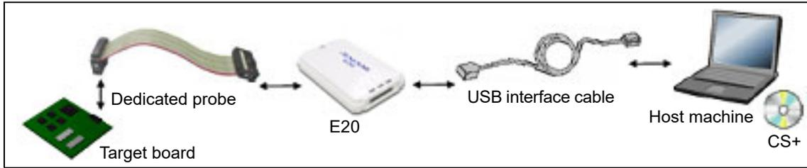
**Caution** Only serial communications are supported as the communication method with the target board (JTAG communications is not available).
