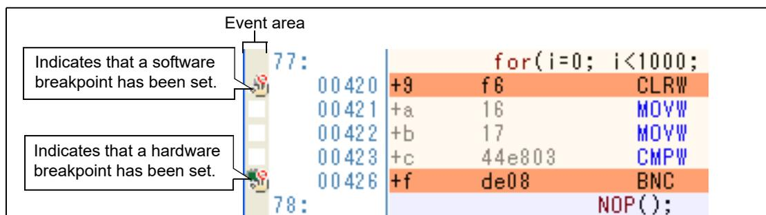
Figure 2.36 Example of Setting Breakpoint in Events Panel
