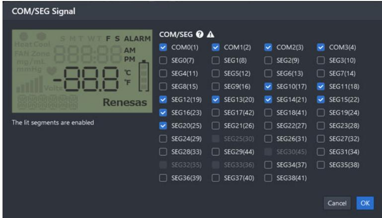
Select the COM and SEG signals to be connected to the LCD panel. Click on the [OK] button to complete the settings.
