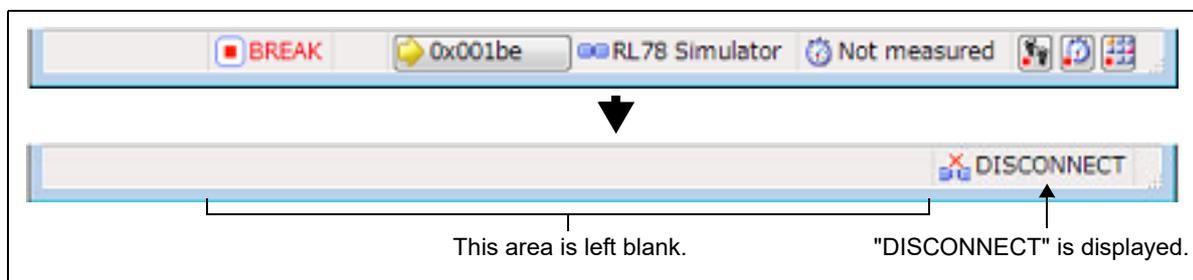
**Caution** The debug tool cannot be disconnected from CS+ while the program is running.
