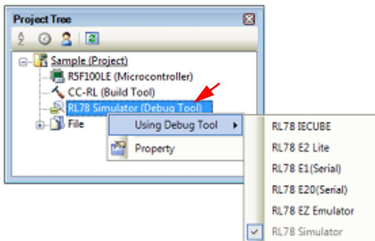
If the [Property panel](#) is already open, click the [RL78 *Debug tool name* (Debug Tool)] node again. The view switches to the Property panel of the selected debug tool.
