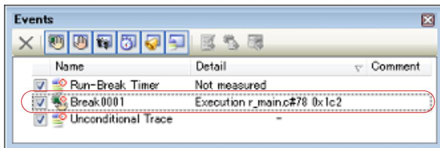
**Caution 1.** Since a breakpoint is set as a break event and managed as a event, restrictions apply to the number of breakpoints that can be simultaneously set. Also see "2.16.7 [Notes for setting events](#)" for details on breakpoints (e.g. limits on the number of enabled events).
