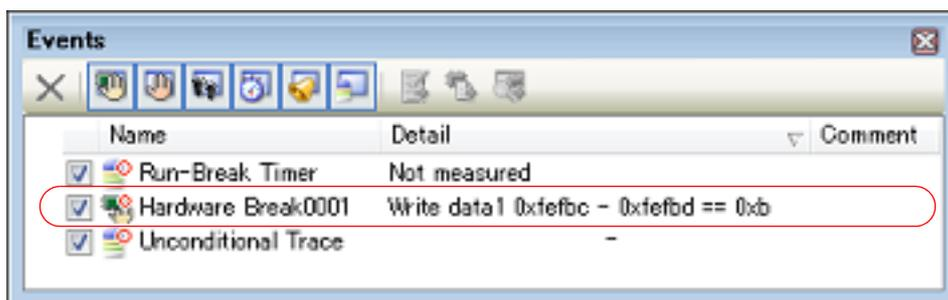
Figure 2.45 Example of Setting Combination Break Event (Access Type) in Events Panel [E1][E20]
