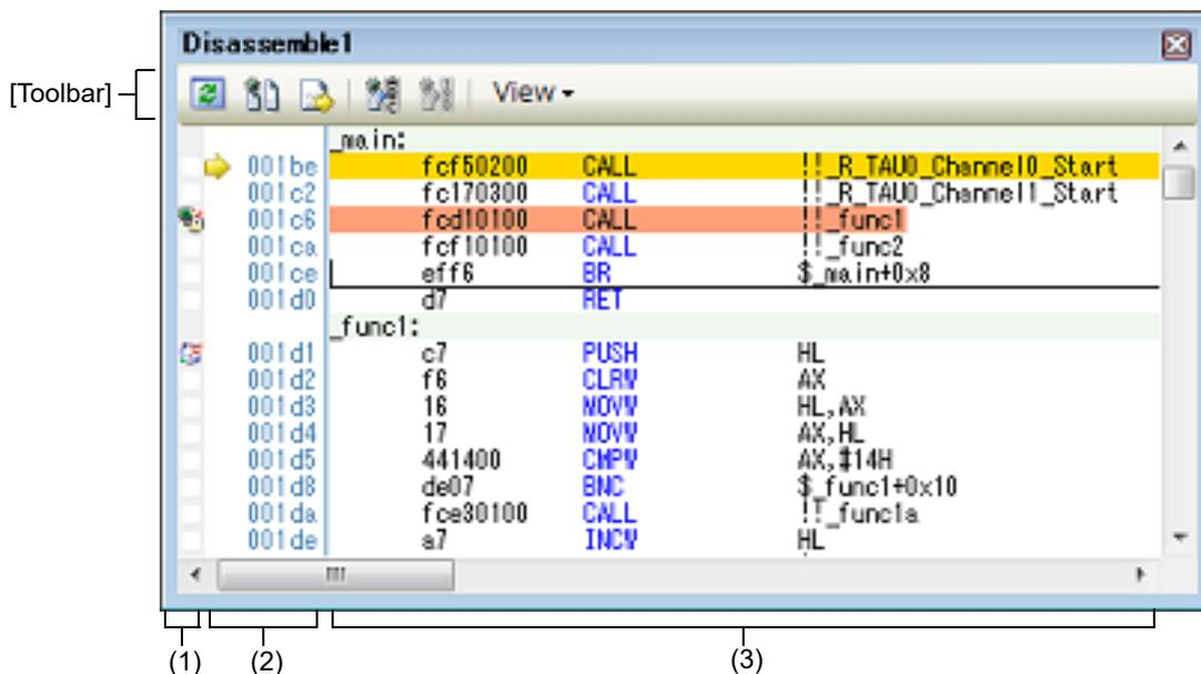
Figure A.9 Disassemble Panel (When Code Coverage Measurement Result Is Displayed)
