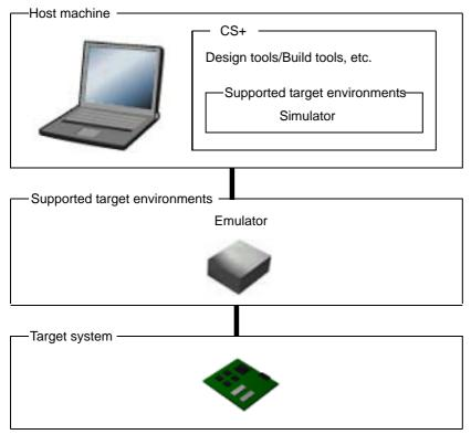
Remark The emulator that can be connected differs depending on the microcontroller used in the project. See "CS+ Integrated Development Environment User's Manual: Debug Tool" for details.
