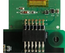
11. Connect the E2 Lite debugger module to the connector marked 'E2 Lite' on the RSK+ using the ribbon cable.
