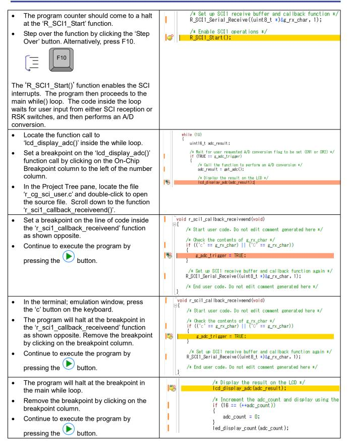
The program proceeds to display the result of the A/D conversion on the LCD and in the terminal window. In addition, the running count of A/D conversions performed is displayed in binary form using LEDs 0-3 on the RSK. Adjust the potentiometer and press any switch on the RSK and an additional A/D conversion will be performed.
