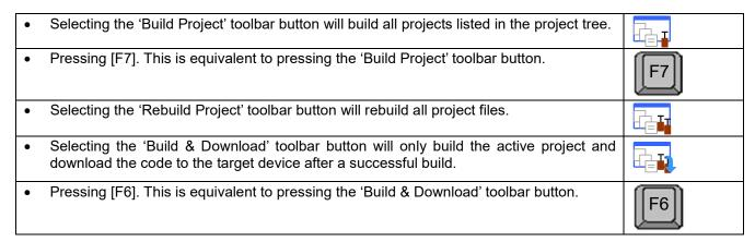
Build the project now by pressing [F7] or pressing one of the build icons as shown above. During the build each stage will be reported in the Output Window. The build will complete with an indication of any errors and warnings encountered during the build.
