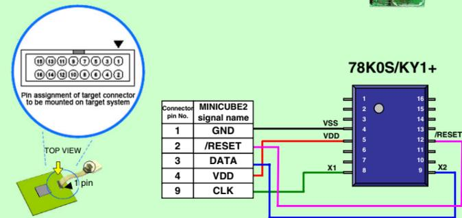
Remark The clock must be supplied from the MINICUBE2 (8MHz). The power can be supplied from it, too. In this case, set Power select switch to "3" or "5". For details, refer to **STEP 4**.
