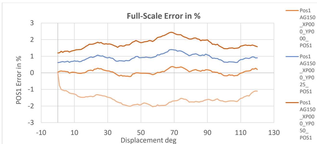
Figure 7. Accuracy with Linearization at 1.5mm Airgap and Effects of Displacement in Y
