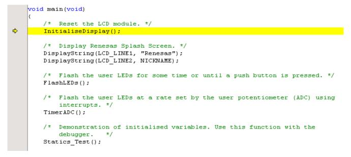
Support for the LCD display is included in the tutorial code. We do not need to be concerned about the details of the LCD interface – except that the interface is write-only and so is not affected if the LCD display is attached or not.
