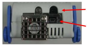
Power supply connector (Connect AC adapter)
