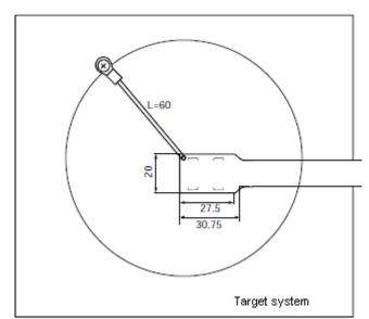
Figure 2-9 Where GND Wire Can Be Connected
