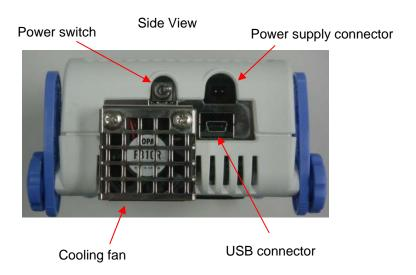
Figure 1-1. Names of Parts of QB-RL78G1A
