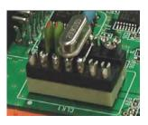
Figure 2-2. Oscillator Shape
