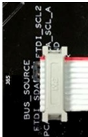
Figure 7. Aardvark Adapter Connection to J65
