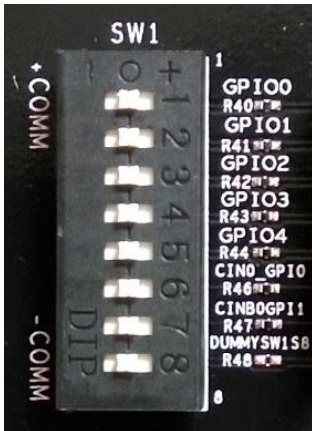
Figure 8. DIP Switch SW1
