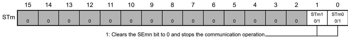
\* Because the ST<sub>m</sub>n bit is a trigger bit, it is cleared immediately when SE<sub>m</sub>n = 0.
