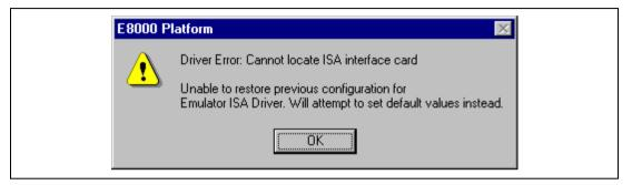
Figure 3.27 Error Message on PC Interface Connection Failure
