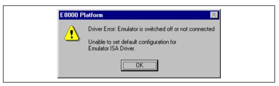
Figure 3.28 Error Message on Emulator Connection Failure
