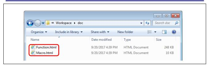
Figure 2.8 Report Files Output by the Report Function of the Code Generator for the e<sup>2</sup> studio
