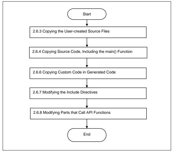
Figure 2.26 Procedure for Porting User-defined Source Code
