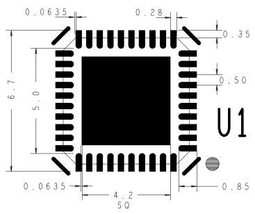
FIGURE 2. QFN LAND PATTERN AND DIMENSIONS (in mm)
