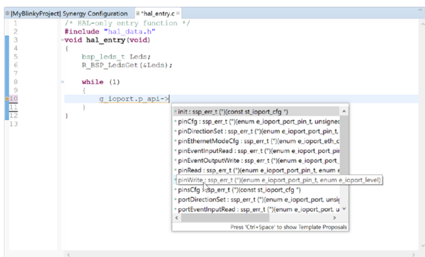
Figure 8-7: Pressing <ctrl>-<space> at a variable or function will activate the code completion feature of the editor
