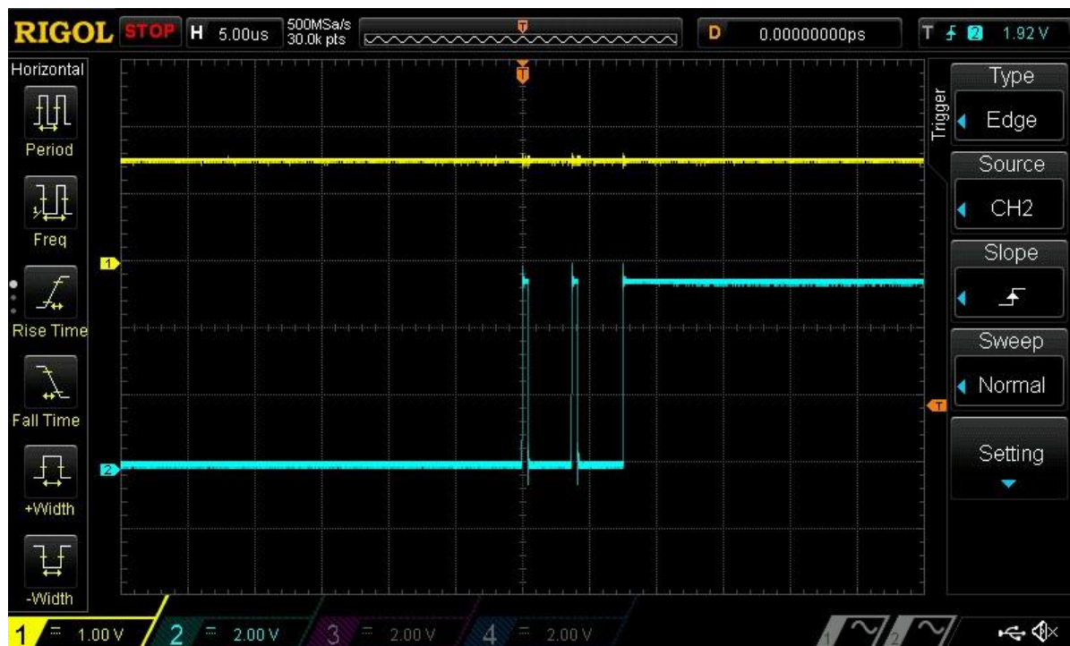
Figure 3: Zoomed ACMP Output during Glitching
