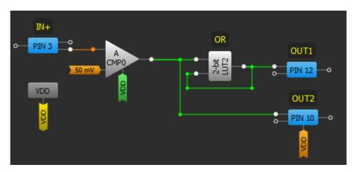
ACMP IN+ is connected to the Ground.
