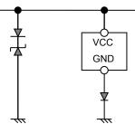
External diode is recommended in order to prevent reverse current toward control logic part at reverse battery condition.
