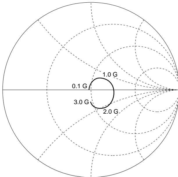
Sパラメータ参考値 (T<sub>A</sub> = +25 )V<sub>CC</sub> = 3.0 V, I<sub>CC</sub> = 6.5 mA
