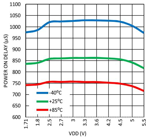
**Figure 51. Maximum Power On Delay vs. VDD,
