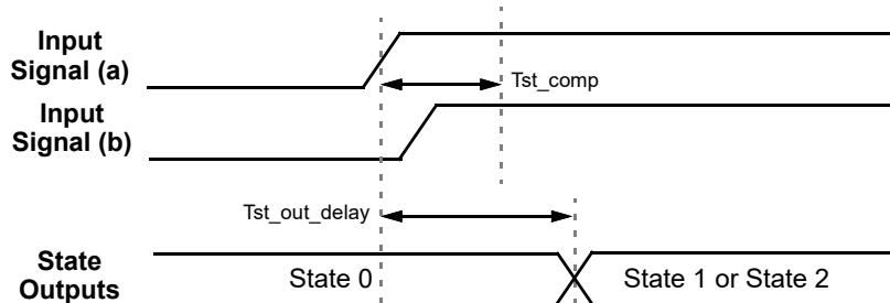
Figure 93. State Transition Timing - Competing Inputs Indeterminate
