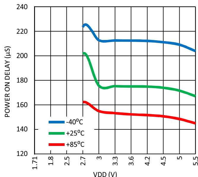
**Figure 50. Maximum Power On Delay vs.  $V_{DD}$ ,
