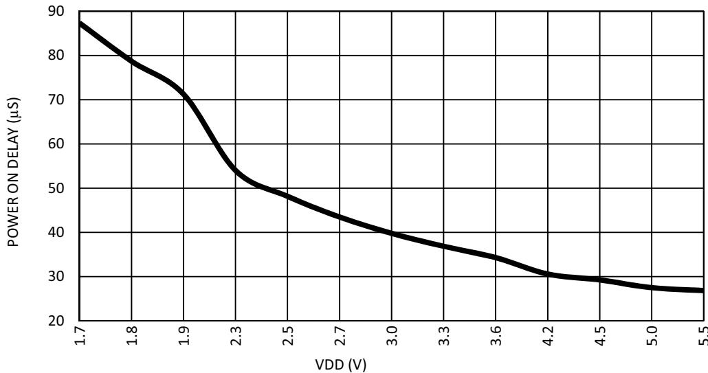
Figure 71. OSC1 (25 MHz) Maximum Power On Delay vs.  $V_{\text{DD}}$  at 85 °C
