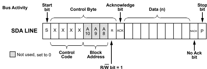
Figure 103. Current Address Read Command,  $\overline{R/W} = 1$
