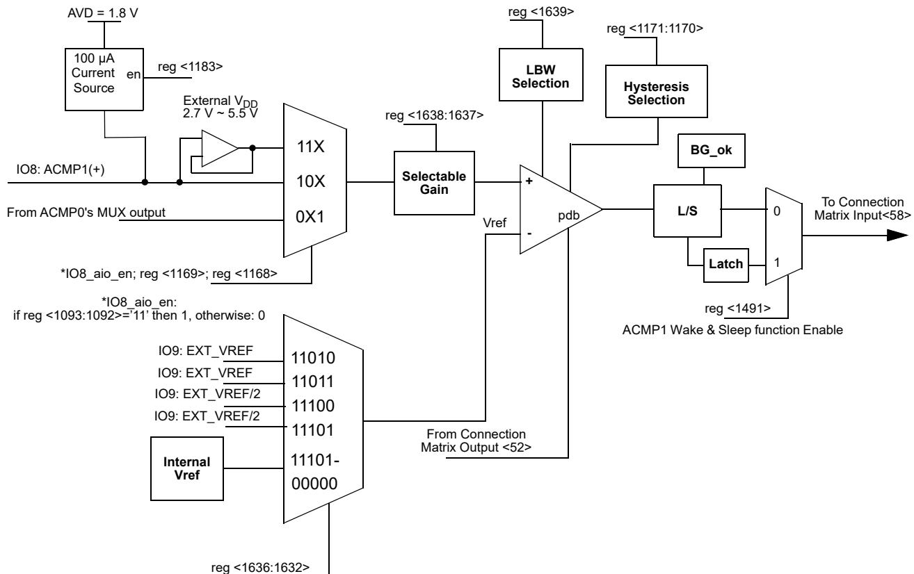
Note: when 100 µA Current Source is enabled input voltage on IO8 should not exceed 1.8 V.
