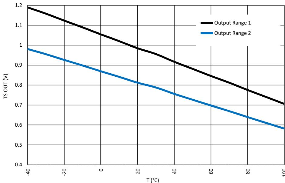
Figure 109. TS Output vs. Temperature,  $V_{DD} = (1.71\dots 5.5)$  V
