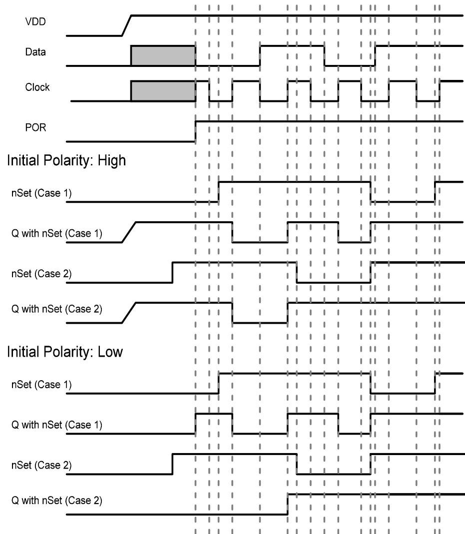
Figure 27. DFF Polarity Operations with nSet
