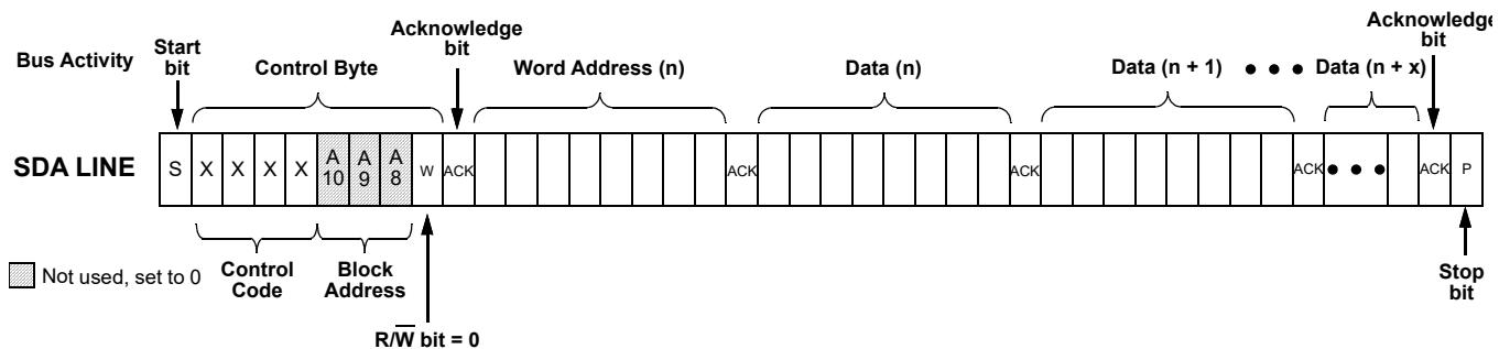
Figure 102. Sequential Write Command,  $\overline{R/W} = 0$
