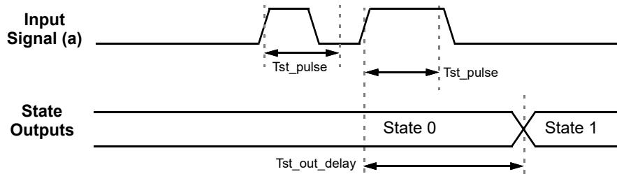
Figure 91. State Transition Pulse Input Timing
