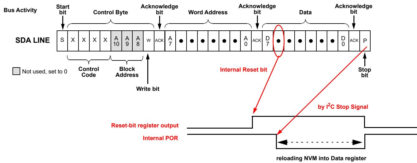
Figure 107. Reset Command Timing
