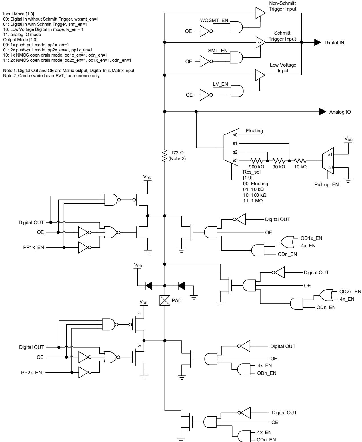
Figure 5. Matrix OE IO 4X Drive Structure Diagram
