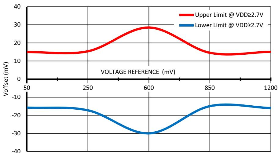
**Figure 53. Typical Buffer Input Voltage Offset vs. Voltage Reference at  $T = (-40 \dots +85)^\circ\text{C}$ ,
