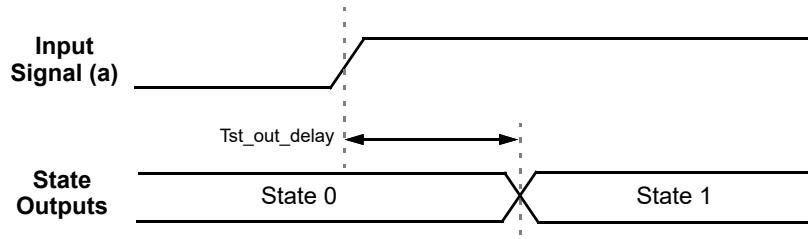
Figure 87. State Transition Timing
