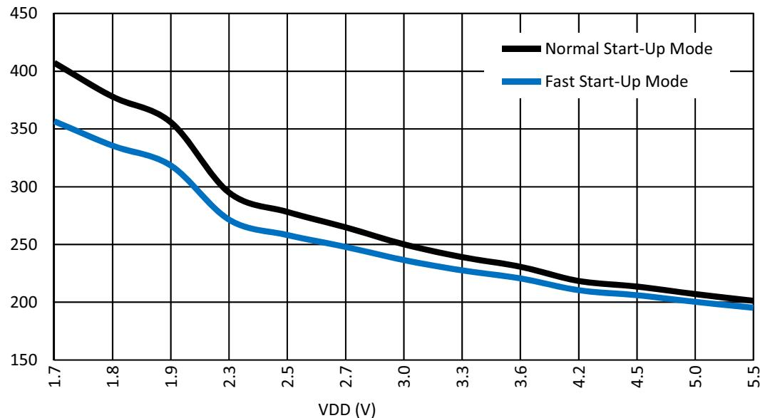
Figure 69. RC Oscillator Maximum Power On Delay vs. V<sub>DD</sub> at room temperature, OSC0 = 2 MHz
