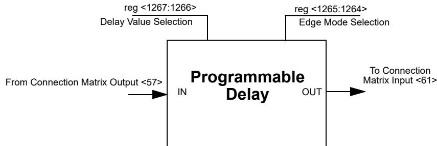
Figure 59. Programmable Delay
