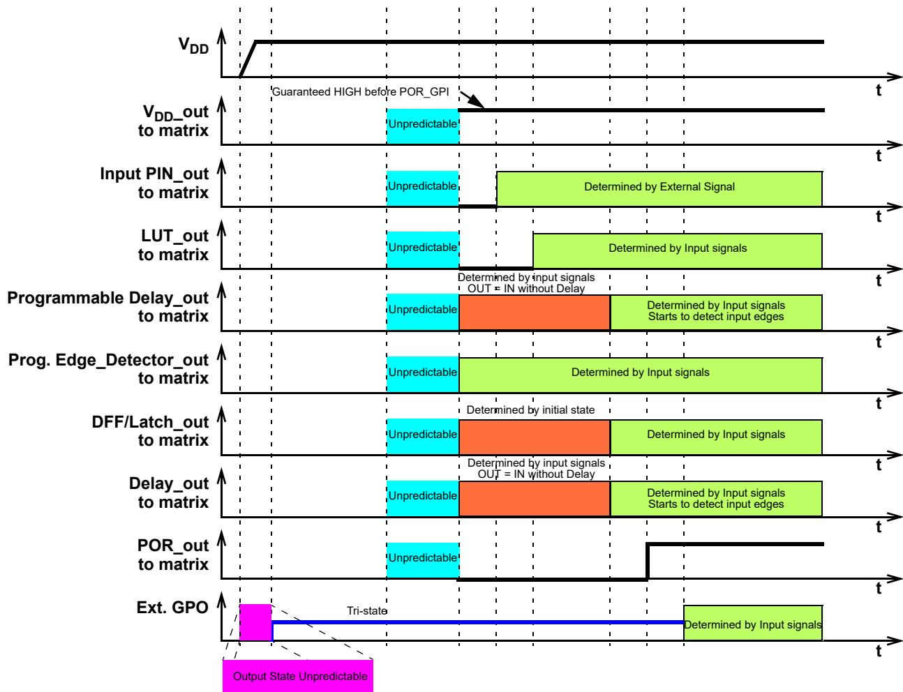
Figure 78. Internal Macrocell States during POR sequence
