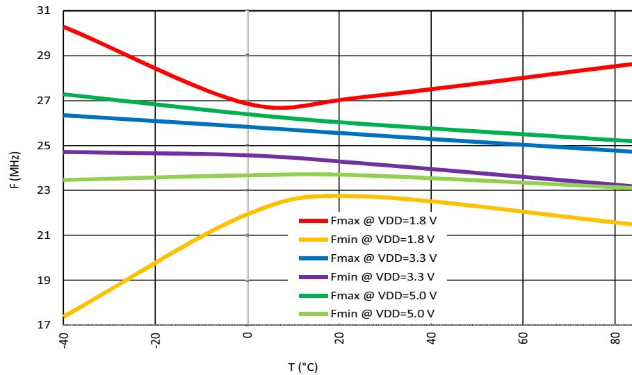
**Figure 74. OSC1 (25 MHz) Frequency vs. Temperature**
