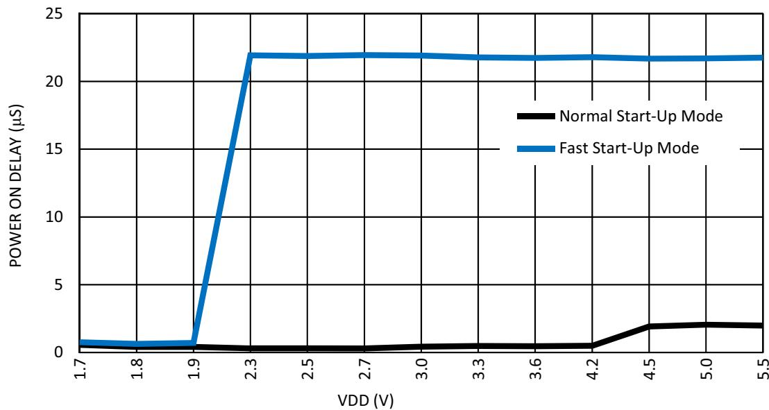
Figure 70. RC Oscillator Maximum Power On Delay vs.  $V_{\text{DD}}$  at 85 °C, OSC0 = 25 kHz
