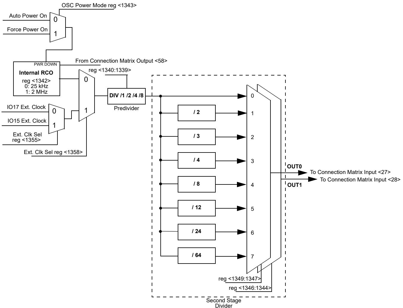
Figure 66. 25 kHz / 2 MHz RC OSC Block Diagram
