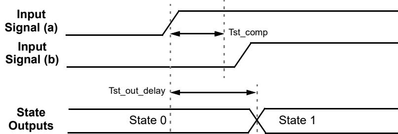
Figure 94. State Transition Timing - Competing Inputs Determinable
