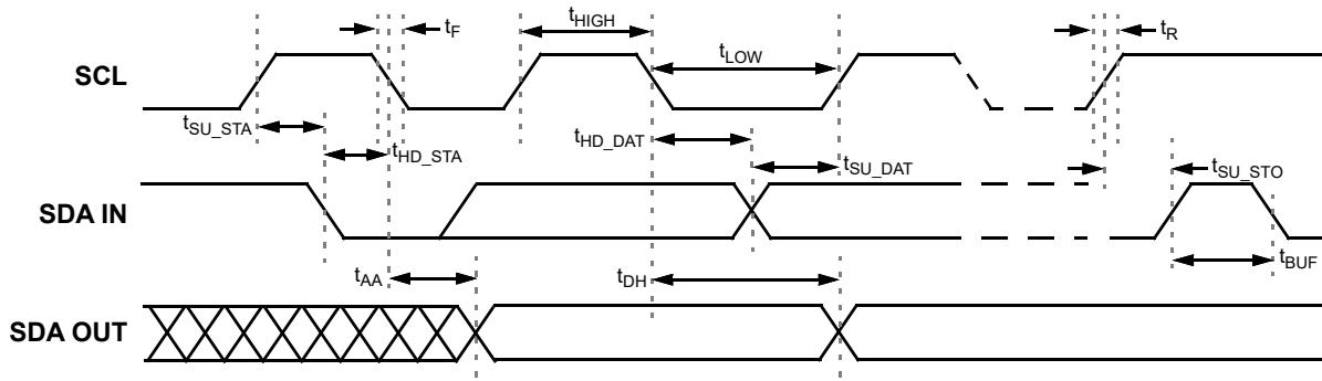
Figure 100. I<sup>2</sup>C General Timing Characteristics
