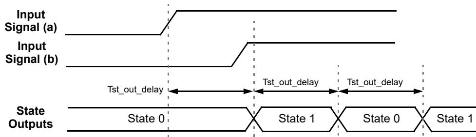
**Figure 98. State Transition - Closed Cycling Timing**
