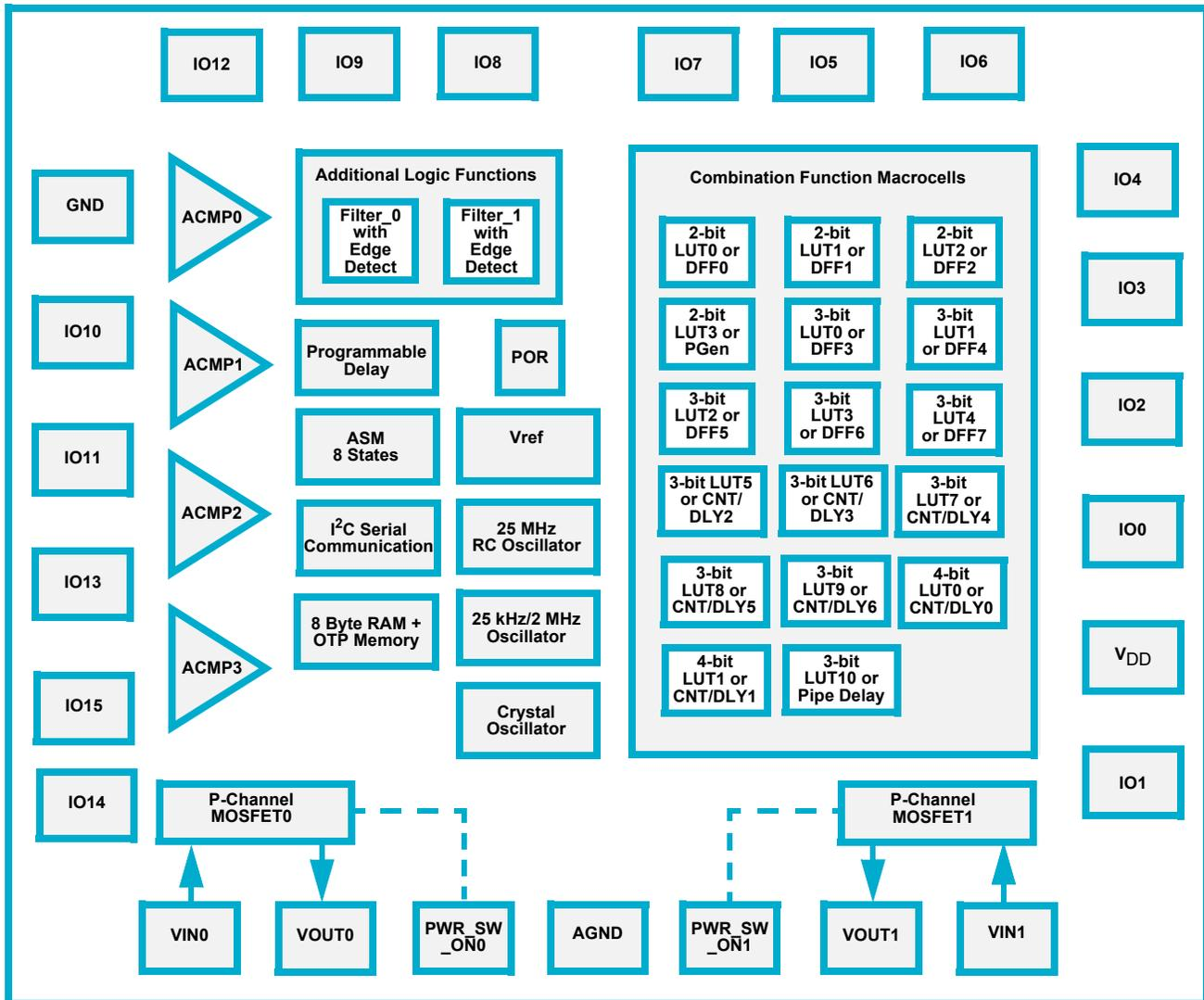
Figure 1: Block Diagram
