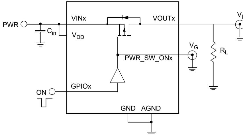
Figure 105: Test Circuit for Typical Switching Waveforms
