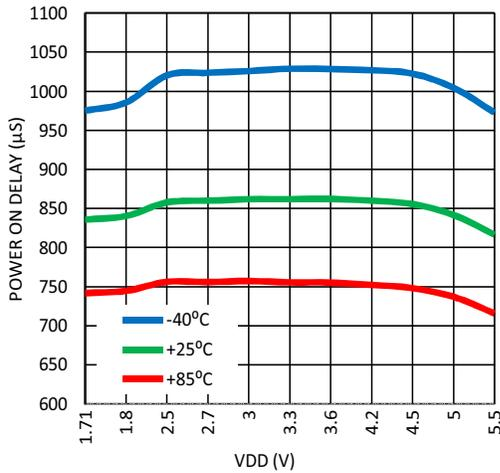
Figure 45: Max. Power-On Delay vs. V<sub>DD</sub>, BG = 550 μs
