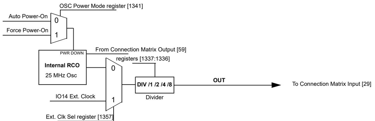
Figure 61: 25 MHz RC OSC Block Diagram
