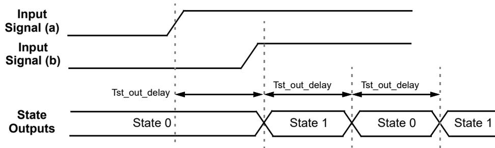
Figure 92: State Transition - Closed Cycling Timing
