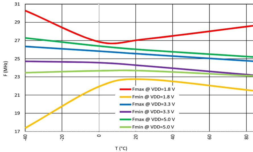
Figure 68: Oscillator Frequency vs. Temperature, OSC1 = 25 MHz
