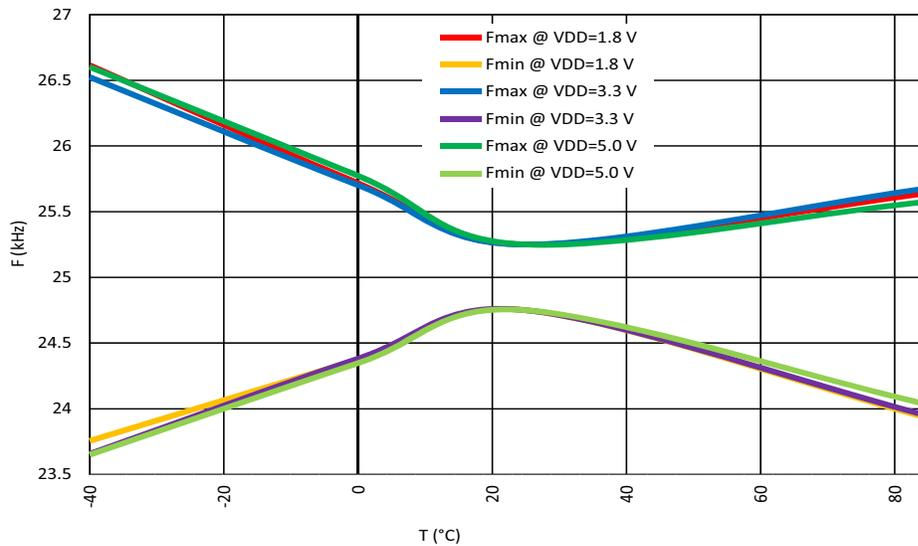
Figure 67: Oscillator Frequency vs. Temperature, OSC0 = 25 kHz
