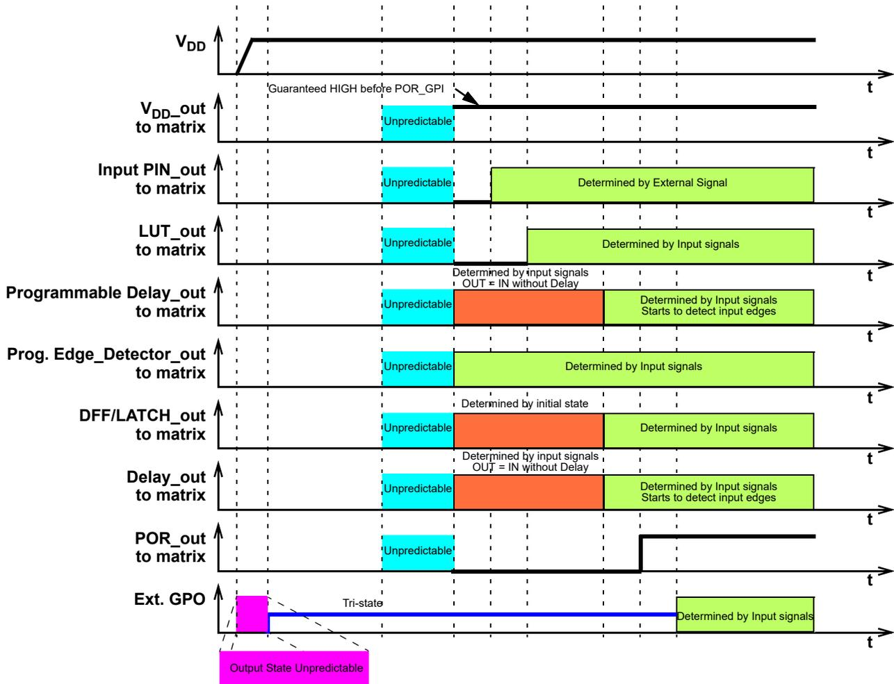
Figure 72: Internal Macrocell States during POR Sequence
