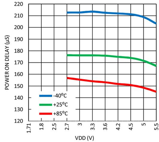
Figure 46: Max. Power-On Delay vs. V<sub>DD</sub>, BG = 100 μs
