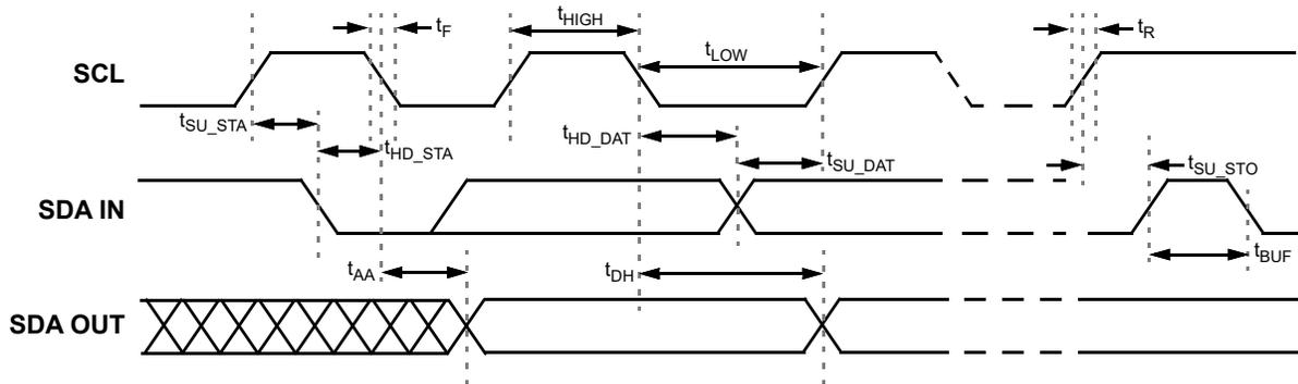
Figure 94: I<sup>2</sup>C General Timing Characteristics
