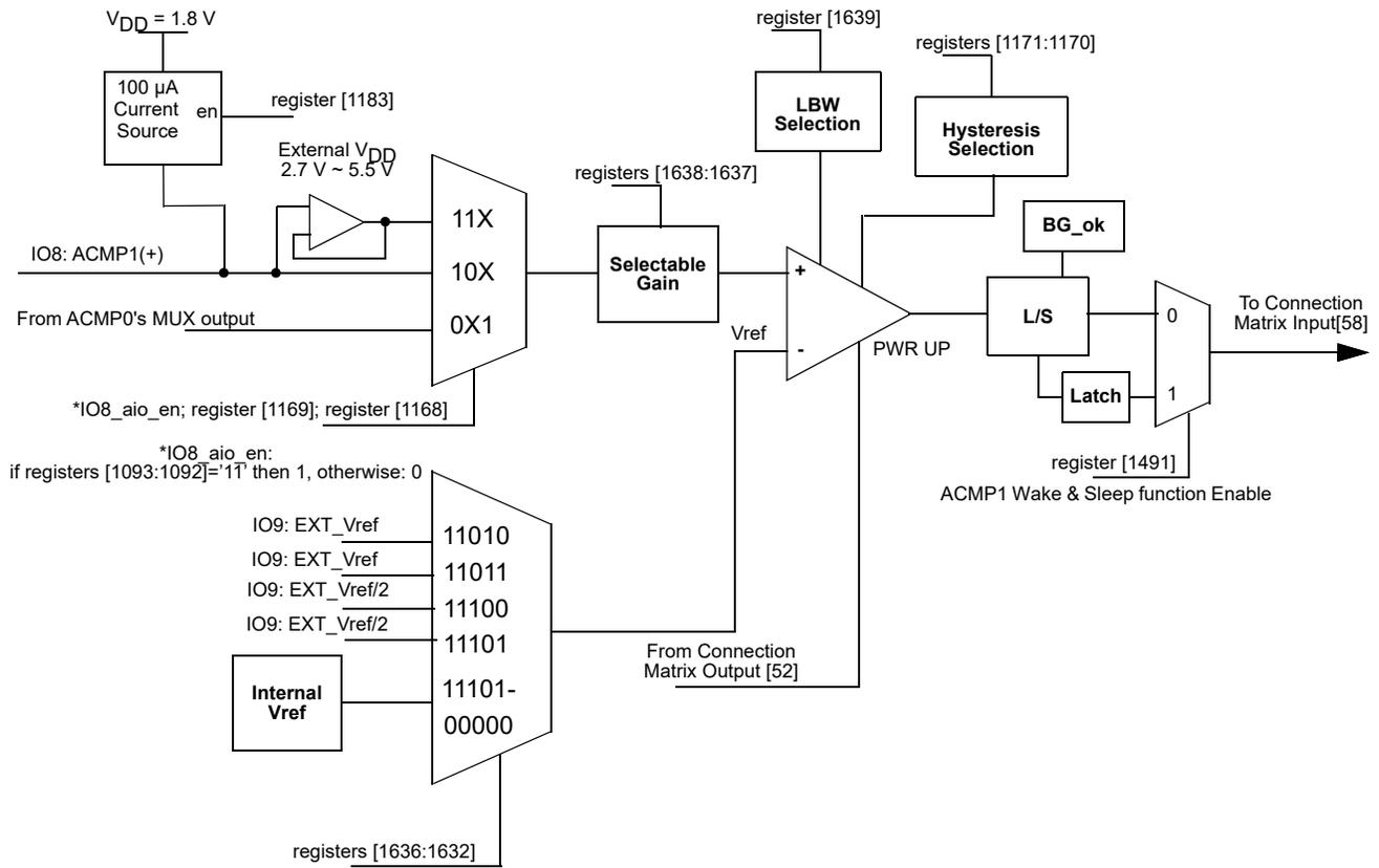
Note: when 100 μA Current Source is enabled input voltage on IO8 should not exceed 1.8 V.
