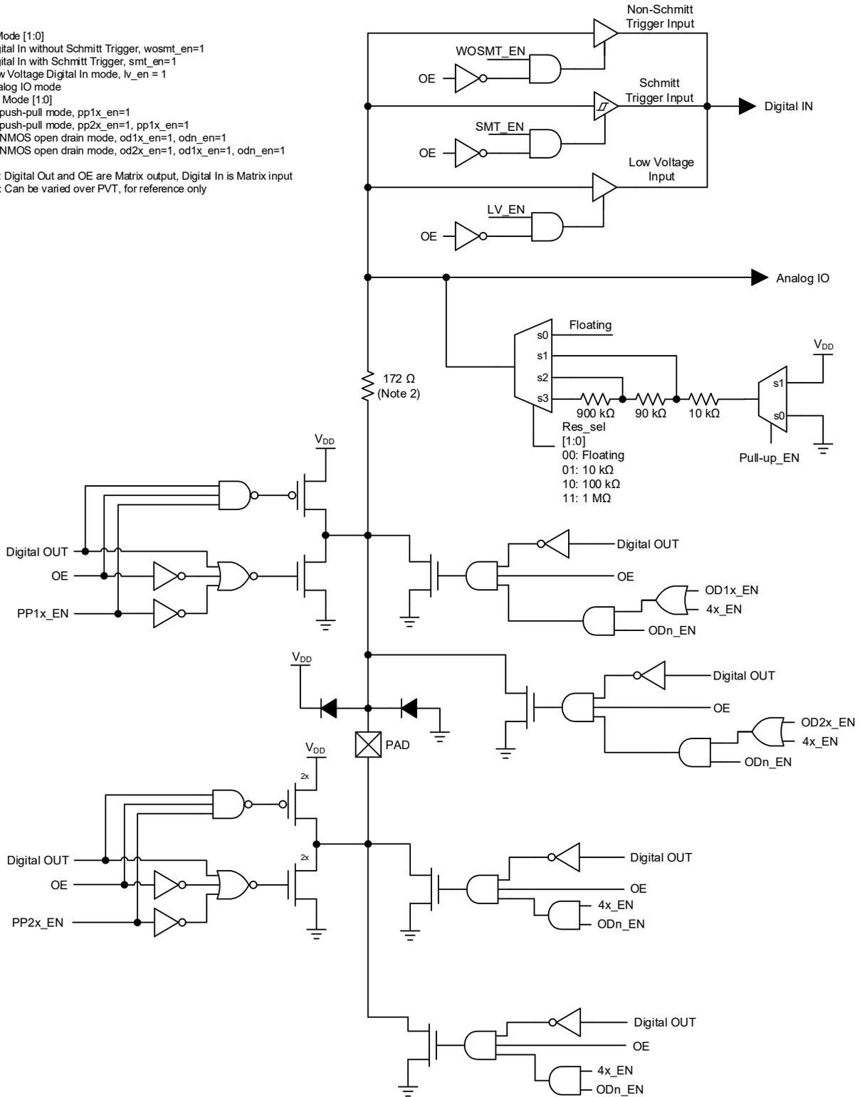
Figure 6: Matrix OE IO 4X Drive Structure Diagram
