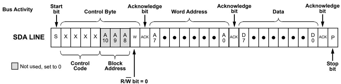
Figure 95: Byte Write Command, R/W = 0
