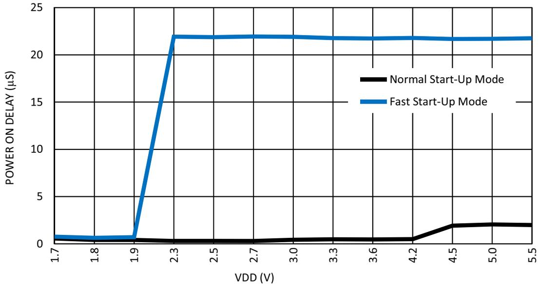
Figure 64: Oscillator Maximum Power-On Delay vs. V<sub>DD</sub> at T = 25 °C, OSC0 = 25 kHz
