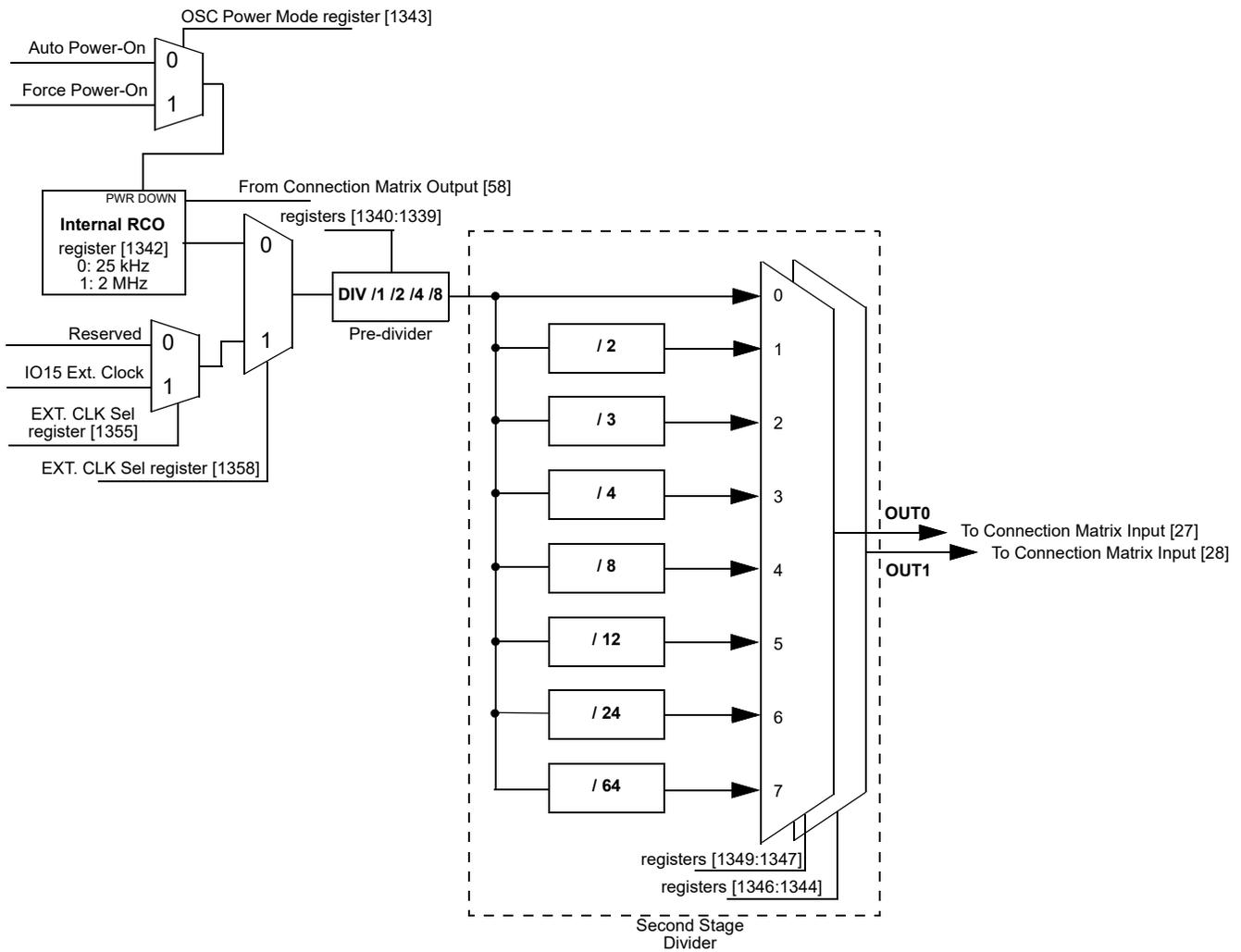
Figure 60: 25 kHz/2 MHz RC OSC Block Diagram
