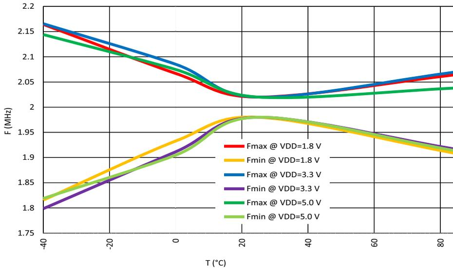
Figure 66: Oscillator Frequency vs. Temperature, OSC0 = 2 MHz
