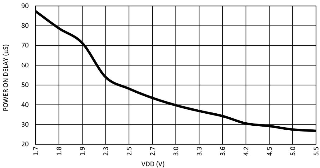
Figure 65: Oscillator Maximum Power-On Delay vs. V<sub>DD</sub> at T = 25 °C, OSC1 = 25 MHz
