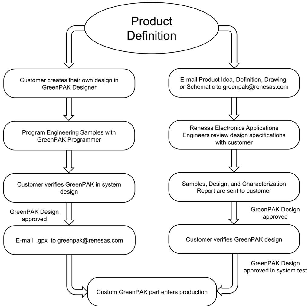
Figure 2: Steps to Create a Custom GreenPAK Device
