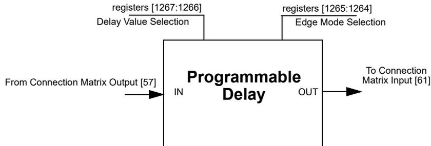
Figure 53: Programmable Delay
