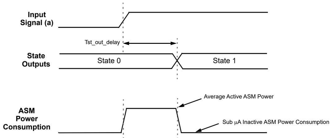
Figure 83: State Transition Timing and Power Consumption
