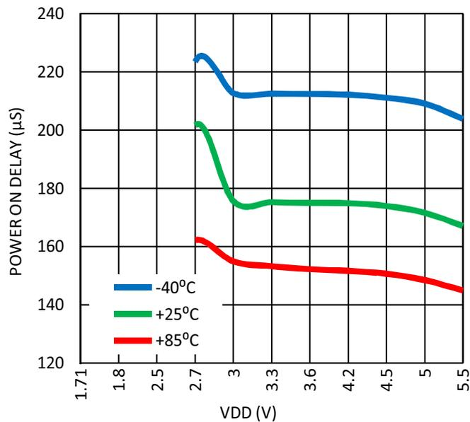
Figure 44: Maximum Power-On Delay vs.  $V_{DD}$ , BG = Auto-delay.
