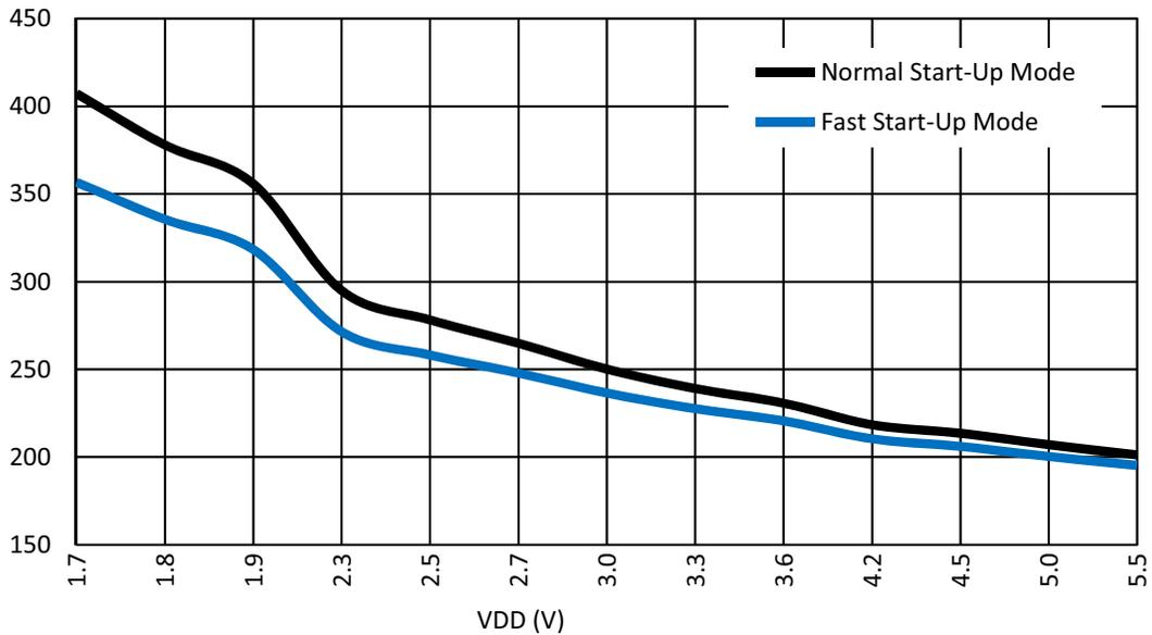
Figure 63: Oscillator Maximum Power-On Delay vs. V<sub>DD</sub> at T = 25 °C, OSC0 = 2 MHz
