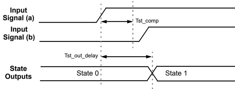
Figure 88: State Transition Timing - Competing Inputs Determinable
