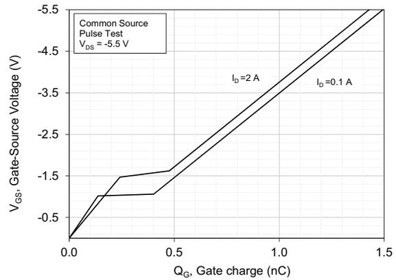
Figure 122: Typical Gate Charge vs. Gate-Source Voltage
