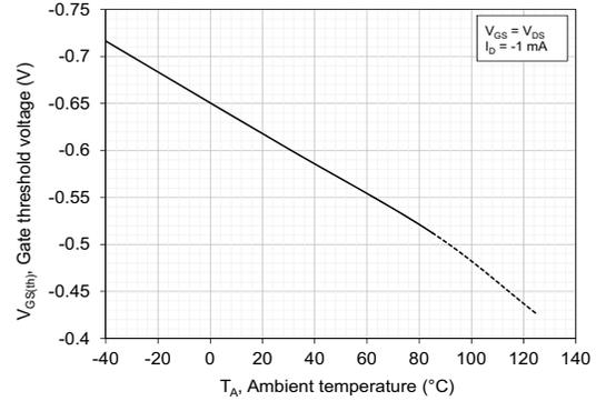
Figure 116: Gate Threshold Voltage vs Ambient Temperature
