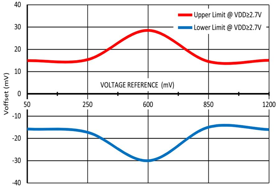
Note: Buffer Bandwidth = 1 kHz,  $V_{\text{phys}} = 0 \text{ mV}$ , Gain = 1,  $T = -40 \text{ }^\circ\text{C}$  to  $+85 \text{ }^\circ\text{C}$
