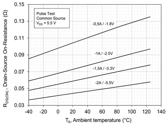
Figure 111: Typical Drain-Source On-Resistance vs. Ambient Temperature
