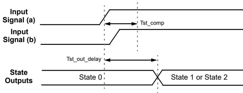
Figure 87: State Transition Timing - Competing Inputs Indeterminate
