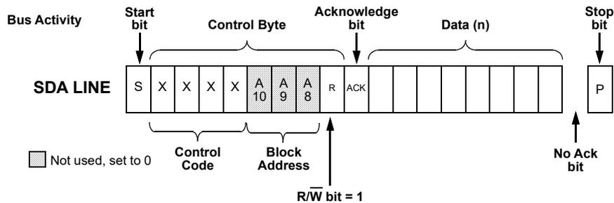
Figure 97: Current Address Read Command,  $\overline{R/W} = 1$
