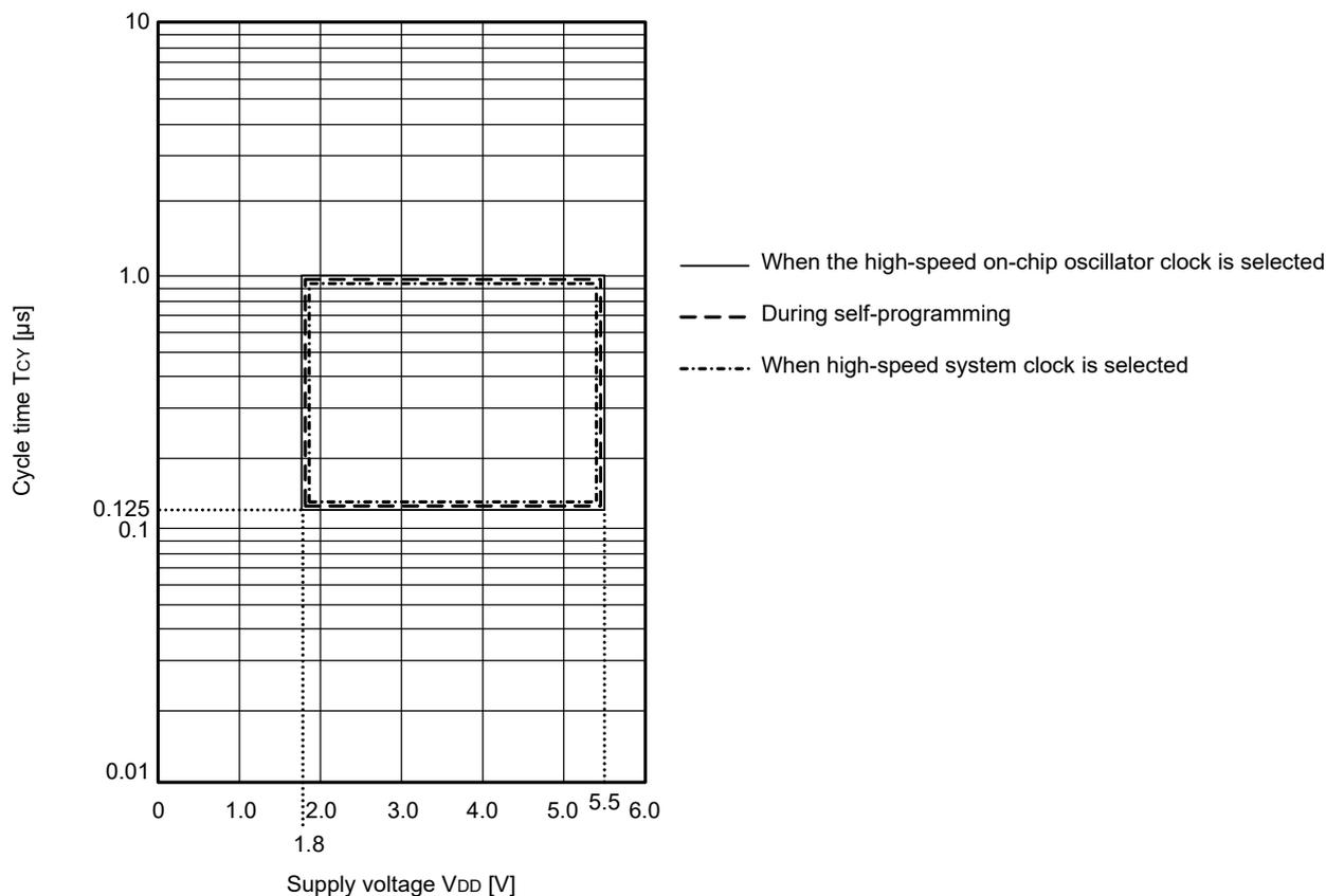
T<sub>CY</sub> vs V<sub>DD</sub> (LV (low-voltage main) mode)
