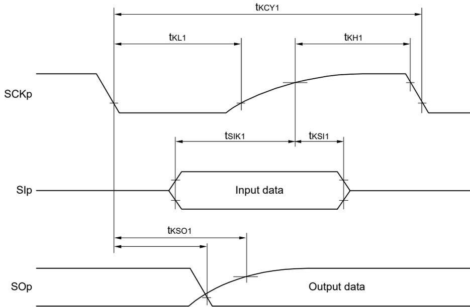
**Simplified SPI (CSI) mode serial transfer timing (master mode) (during communication at different potential)
