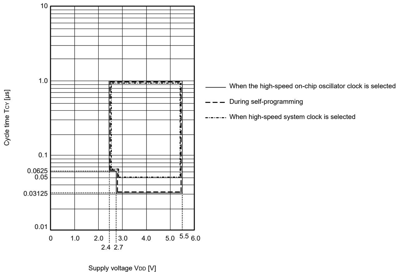
T<sub>CY</sub> vs V<sub>DD</sub> (LS (low-speed main) mode)
