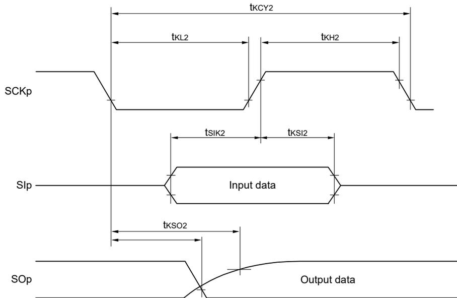
**Simplified SPI (CSI) mode serial transfer timing (slave mode) (during communication at different potential)
