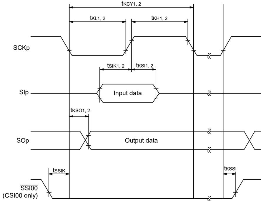
**Simplified SPI (CSI) mode serial transfer timing (during communication at same potential)**
