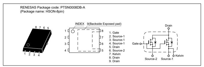
Remark: Strong electric field, when exposed to this device, can cause destruction of the gate oxide and ultimately degrade the device operation. Step must be taken to stop generation of static electricity as much as possible, and quicky dissipate it once, when it has occurred.
