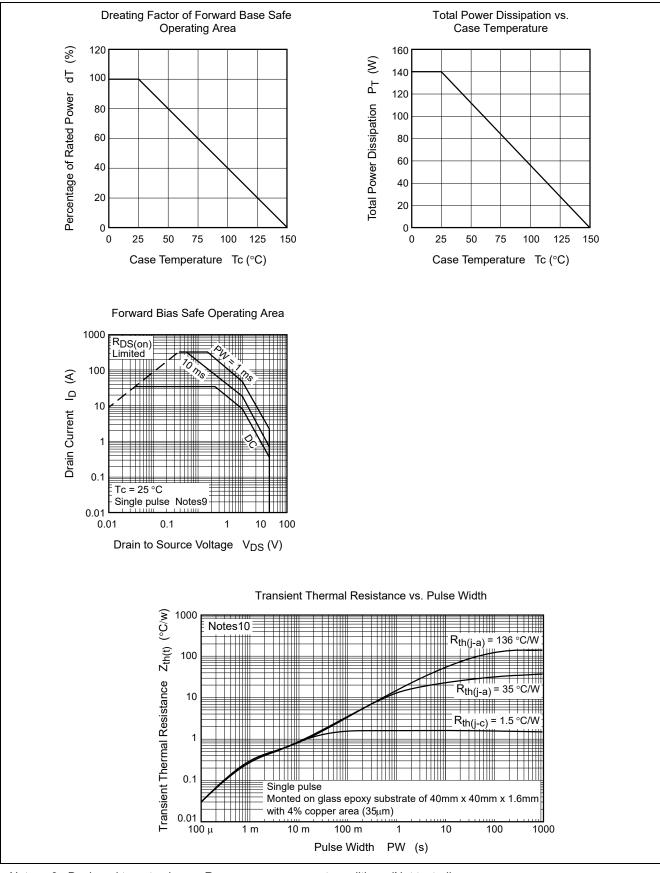
Notes: 9. Designed target value on Renesas measurement condition. (Not tested) Renesas recommends that operating conditions are designed according to a document "Power MOS FET • IGBT Attention of Handling Semiconductor Devices".
