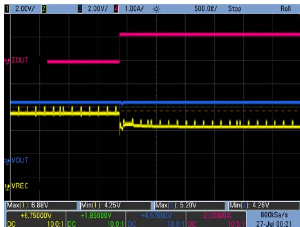
Figure 11. Load Transient: V_{OUT} = 5V , 0A \rightarrow 1.2A
