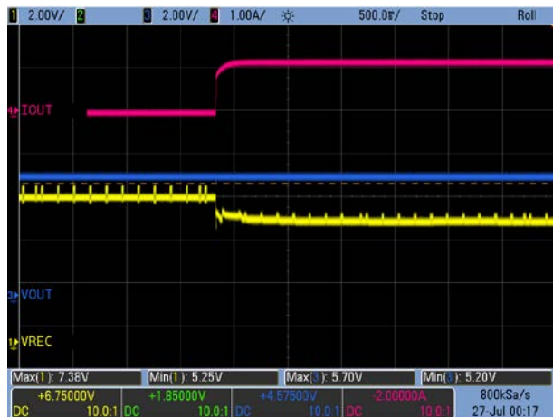
Figure 11. Load Transient: V_{OUT} = 5V , 0A \rightarrow 1.2A
