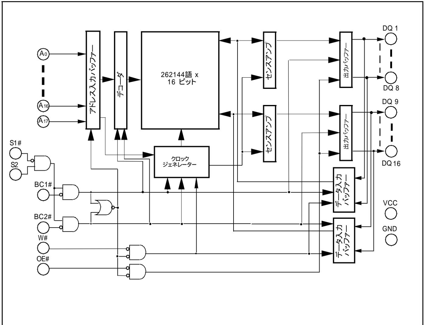
**M5M5V416CWG - 55HI, - 70HI****4194304-BIT (262144-WORD BY 16-BIT) CMOS STATIC RAM**
