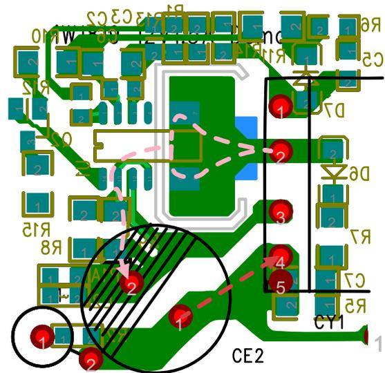
Figure 10.8b : Layout of Primary-Side Power Path
