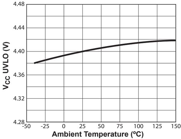
Figure 8.1 : V<sub>CC</sub> UVLO vs. Temperature
