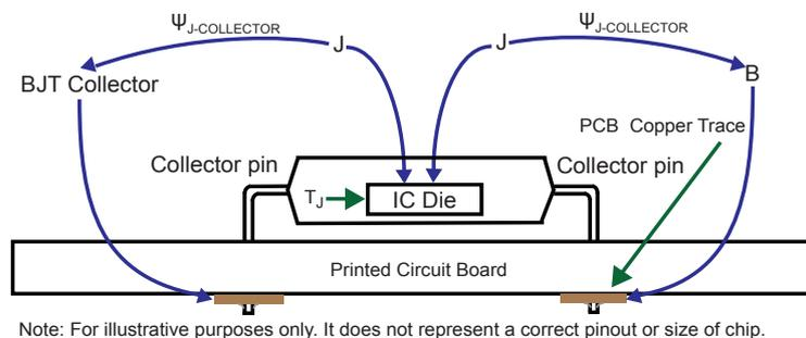
Figure 10.5 : Thermal Resistance
