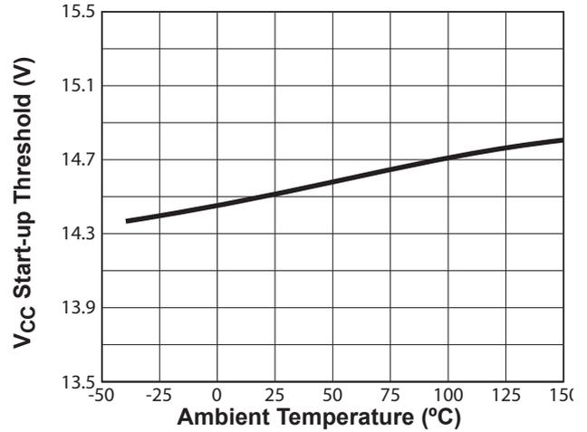
Figure 8.2 : V<sub>CC</sub> Start-up Threshold vs. Temperature
