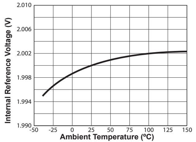
Figure 8.5 : Internal Reference Voltage vs. Temperature
