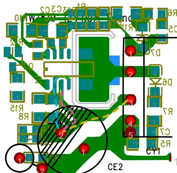
Figure 10.11b : IC and Transformer Ground Layout Path
