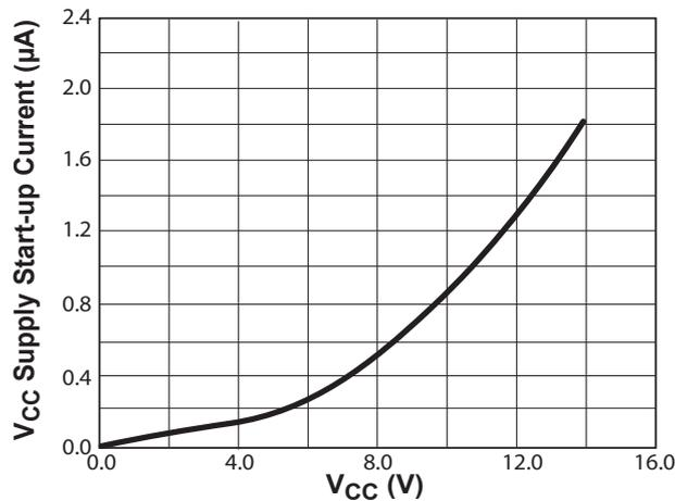
Figure 8.4 : V<sub>CC</sub> Supply Start-up Current vs. V<sub>CC</sub>
