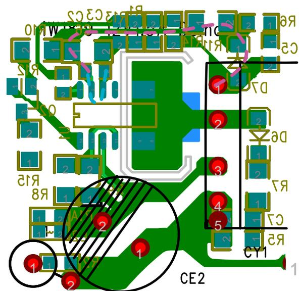
Figure 10.13b : IC Power Supply Layout Path
