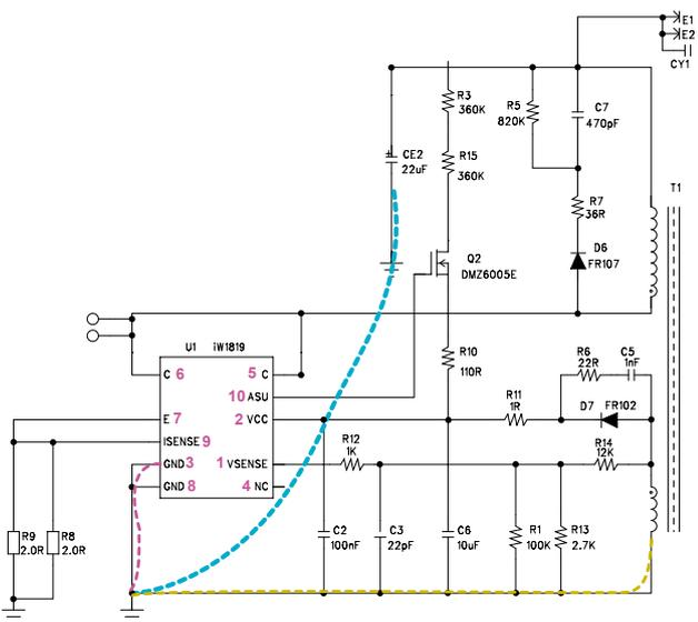
Figure 10.11a : IC and Transformer Ground Path
