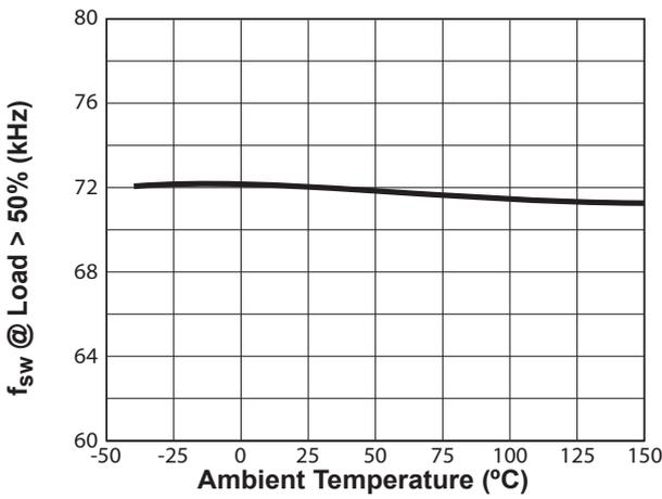
Figure 8.3 : Switching Frequency vs. Temperature<sup>1</sup>
