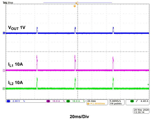
Figure 25. Dual-Phase Waveforms, Burst Mode Waveforms,  $V_{IN} = 48V$ ,  $I_{OUT} = 0.1A$
