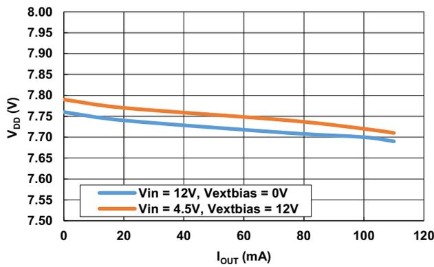
Figure 8. V<sub>DD</sub> Load Regulation at 12V Input
