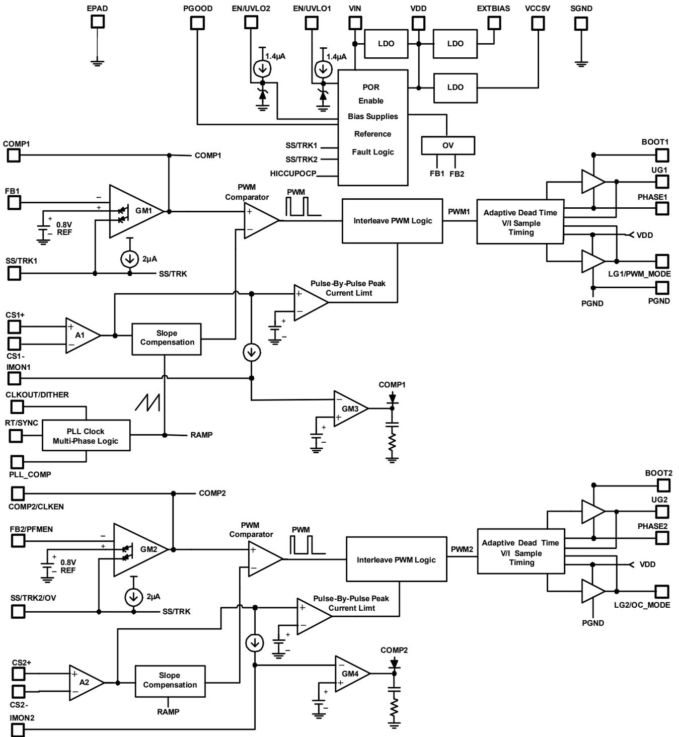
Figure 5. Block Diagram
