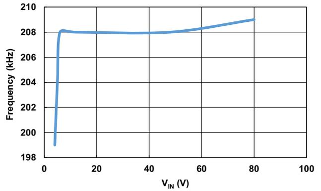
Figure 13. Switching Frequency vs V<sub>IN</sub>, R<sub>T</sub> = 169k
