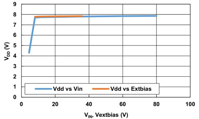
Figure 9. V<sub>DD</sub> Line Regulation at 20mA Load
