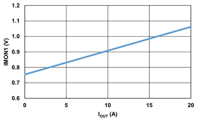
Figure 17. Dual-Phase Output Current I<sub>OUT</sub> (DC) vs IMON1 Pin Voltage, R<sub>S\_out</sub> = 4mΩ, R<sub>IMON1</sub> = 20k
