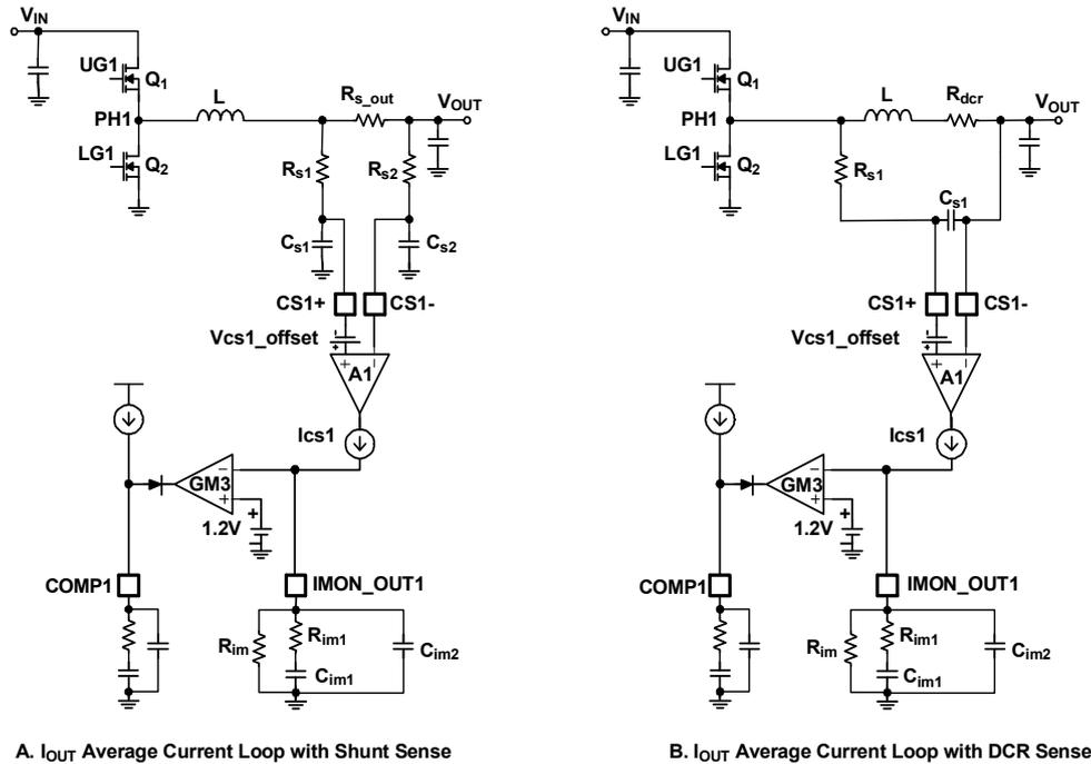
**Figure 39. Output Average Current Monitoring and Regulation Loops**
