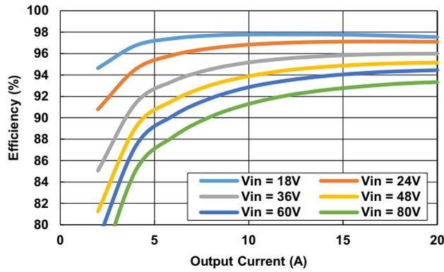
Figure 2. Efficiency ( $V_{OUT} = 12V$ , CC Mode)
