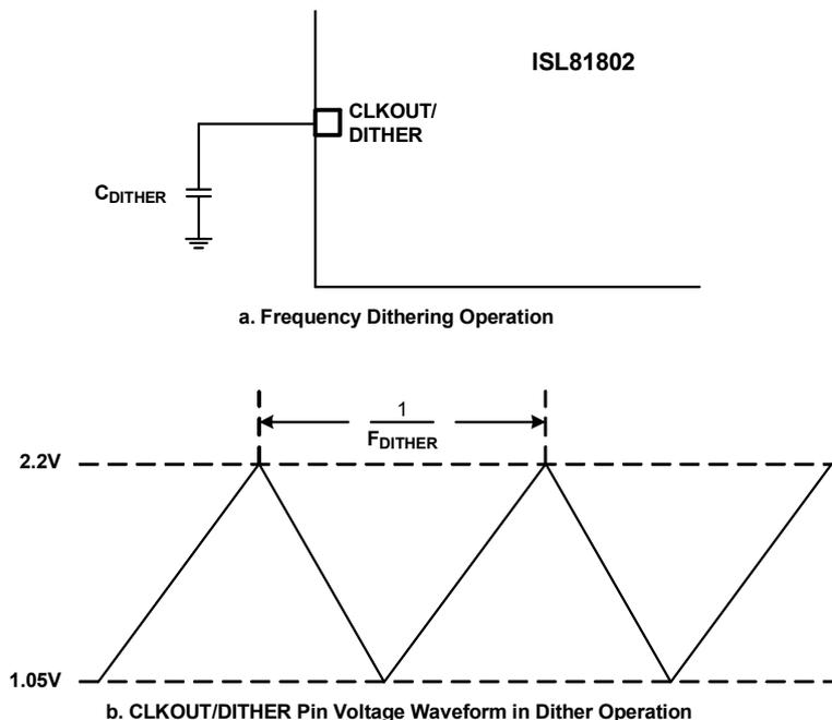
**Figure 42. Frequency Dithering Operation**
