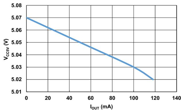
Figure 10. V<sub>CC5V</sub> Load Regulation at 12V<sub>IN</sub>
