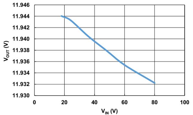
Figure 21. CCM Line Regulation at 20A Load +25°C
