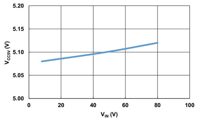
Figure 11. V<sub>CC5V</sub> Line Regulation at 20mA Load
