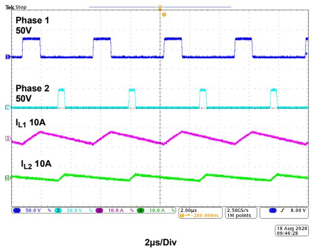
Figure 29. Dual-Output Waveform,  $V_{IN} = 48V$ ,  $V_{OUT1} = 12V$ ,  $V_{OUT2} = 5V$ ,  $I_{OUT1} = 0A$ ,  $I_{OUT2} = 0A$  CCM
