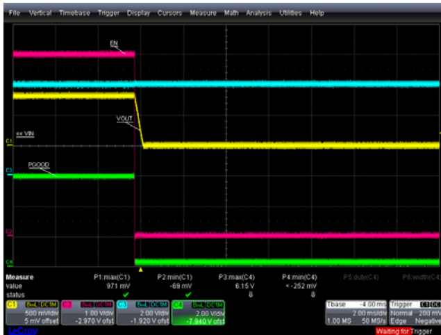
FIGURE 25. POWER-ON AND POWER-OFF, EN = 1 TO 0, +25°C, VIN = 6V, VOUT = 0.8V, IOUT = 0.5A, PGOOD TURN-OFF
