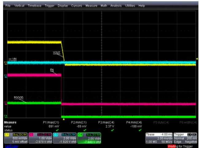
FIGURE 26. POWER-ON AND POWER-OFF, EN = 1 TO 0, +25°C, VIN = 2.2V, VOUT = 0.8V, IOUT = 0.5A, PGOOD TURN-OFF
