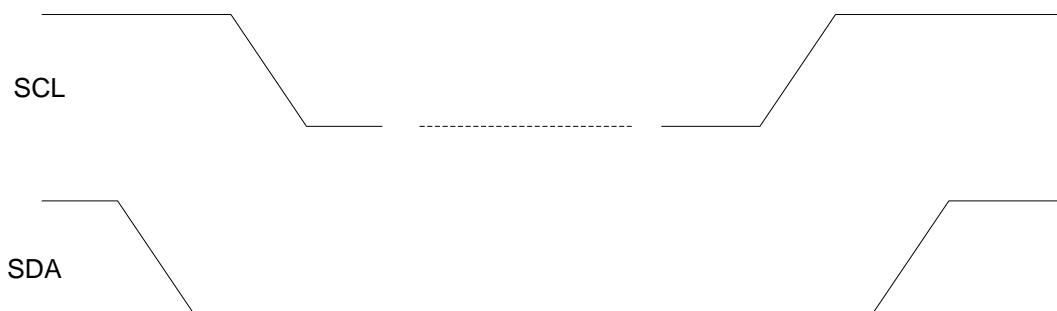
Figure 11: I 2 C START and STOP Condition Timing
