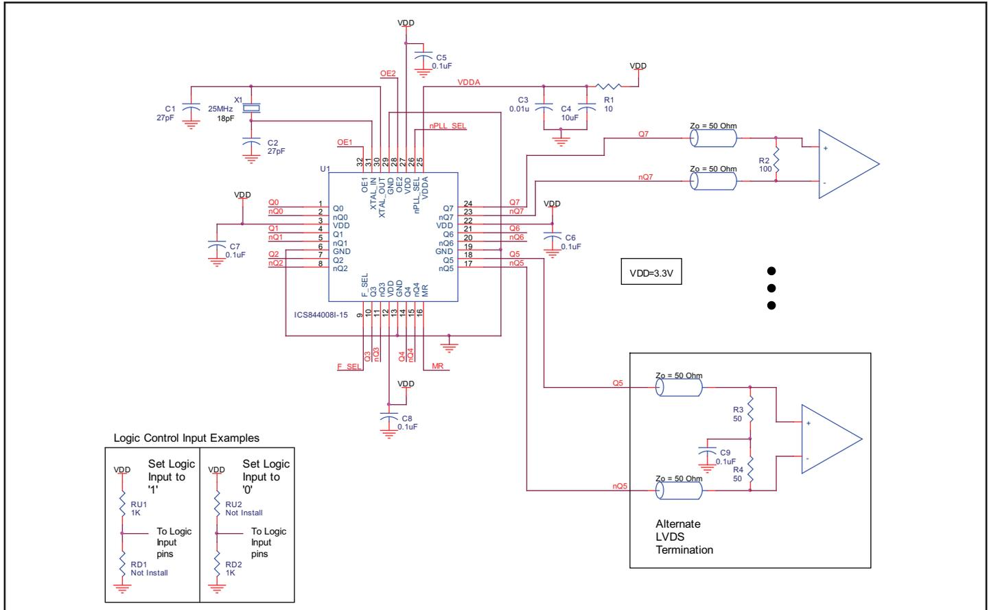
FIGURE 4. 8440081-15 SCHEMATIC EXAMPLE
