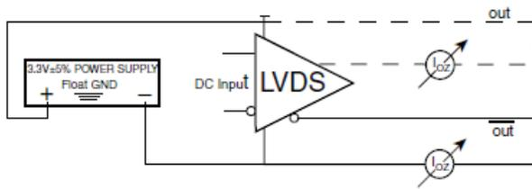
HIGH IMPEDANCE LEAKAGE CURRENT SETUP
