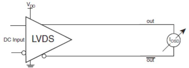
DIFFERENTIAL OUTPUT SHORT CIRCUIT SETUP
