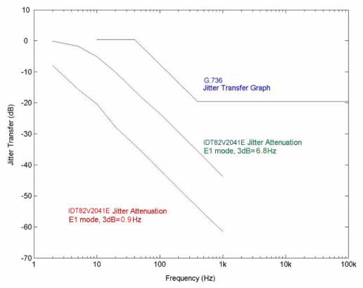
Figure-24 E1 Jitter Transfer Performance
