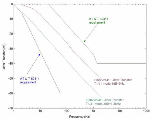
Figure-25 T1/J1 Jitter Transfer Performance
