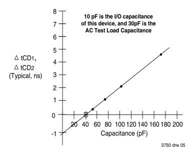
Figure 3. Typical Output Derating (Lumped Capacitive Load).
