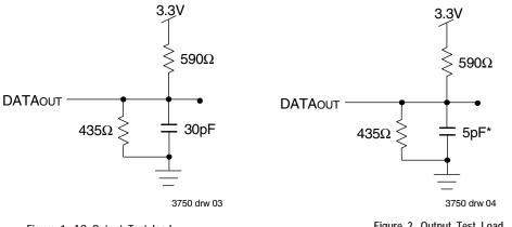
Figure 1. AC Output Test load.
