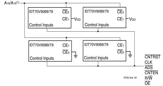
Figure 4. Depth and Width Expansion with IDT70V9089/79
