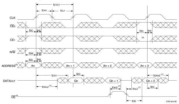
Timing Waveform of Read Cycle for Pipelined Output (FT/PIPE"x" = VIH)<sup>(3,6)</sup>
