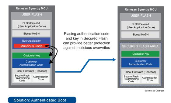
By placing authentication code and key in secured flash, Renesas Synergy's authenticated boot function extends product life.
