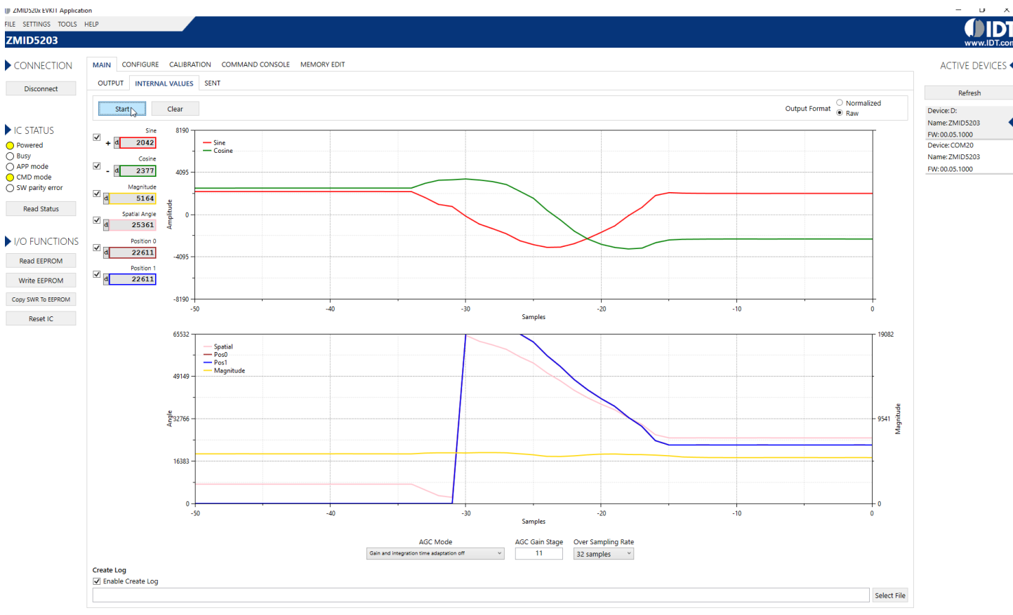
Figure 8. SPA with Non-monotonic Characteristic (with “Jump”)
