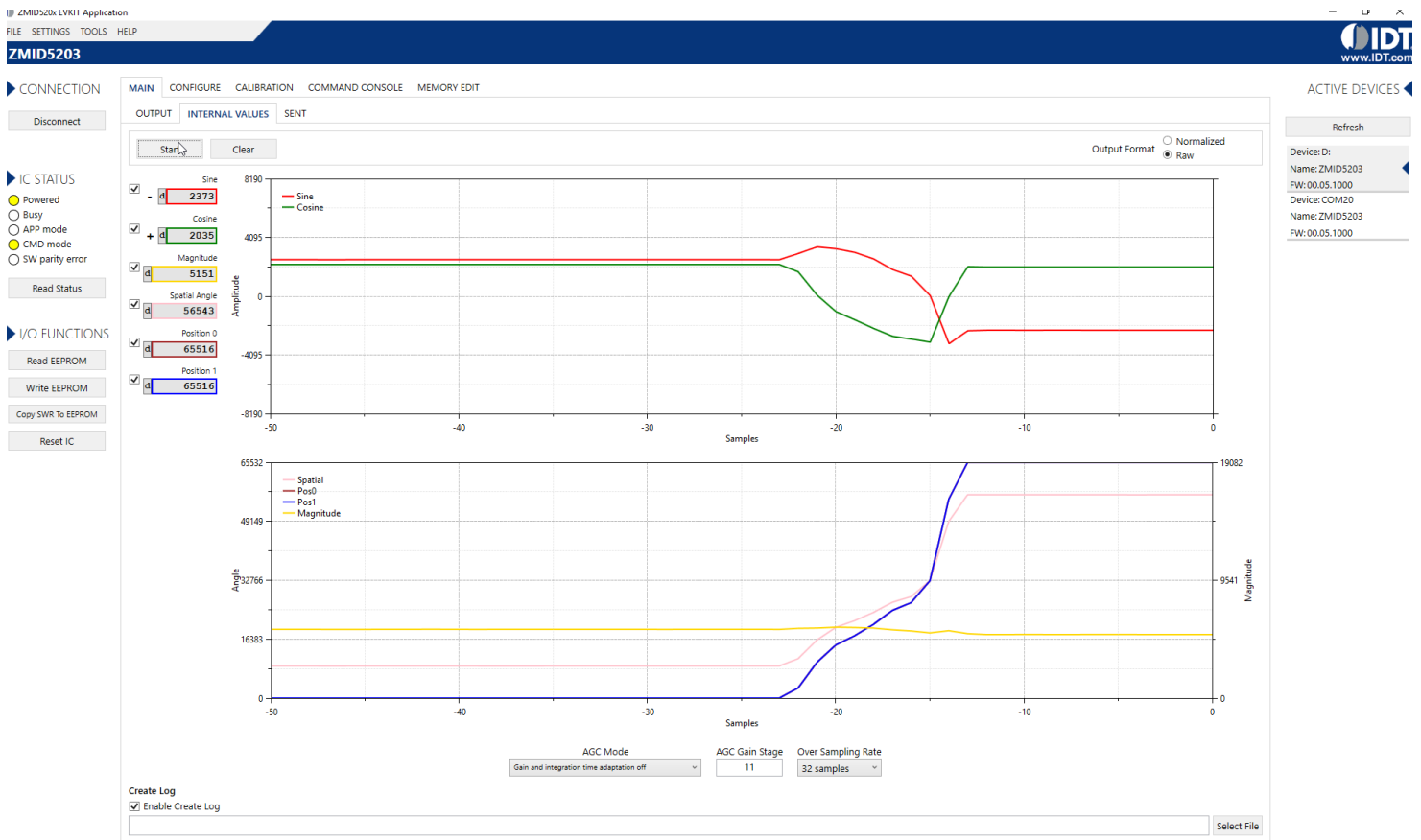
Figure 7. SPA Monotonic Characteristic
