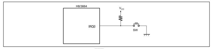
Figure 1 Example of IRQ0 Input Pin Switch Connection
