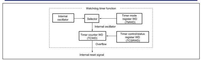
Figure 2.1 Block Diagram of Watchdog Timer Function
