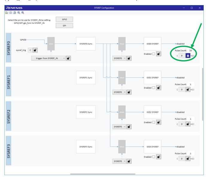
The final step is to enable SYSREF. Select the "Enabled" check box. The SYSREF pulses will generate from IOD0 when GPIO0 transitions from '0' to '1'. Additional pulses will generate with additional GPIO0 toggles.
