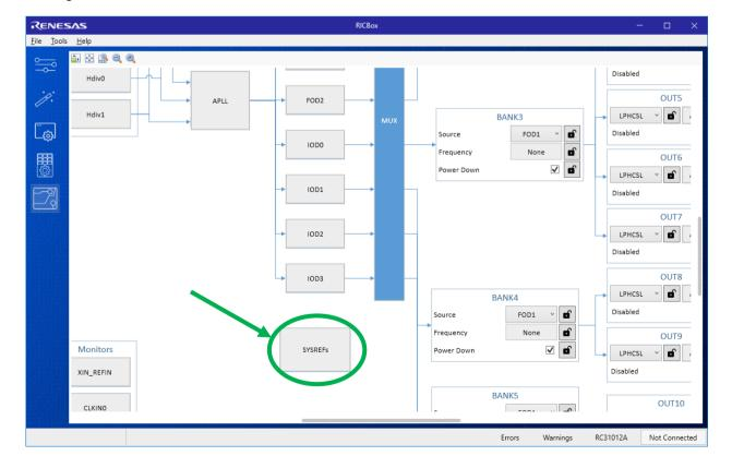
3. Decide how SYSREF0 will be triggered. Trigger from SYSREF\_IN requires defining a GPIO/GPI as a SYSREF\_IN. Trigger from register sysref\_trig uses the respective register field value to transition from '0' to '1'.
