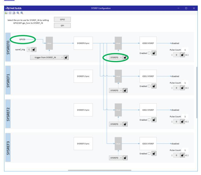
Depending on the SYSREF application, the next step is to set the number of pulses to generate. VC7 can support generating 1 to 256 pulses. To set the pulse count, enter the desired value in the "Pulse Count" (sysref pulse cnt) field. Note that the value entered will result in value + 1 pulses.
